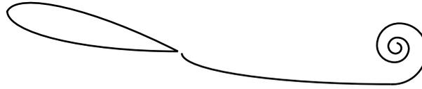
**Figure 2.2.** An impulsive started airfoil sheds a starting vortex
