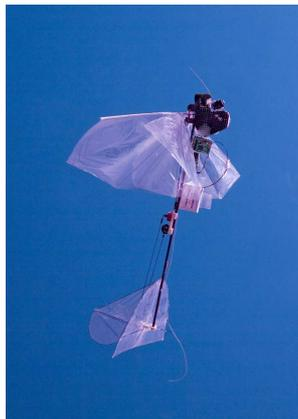
**Figure 3.1.** The flapping MAV DeIFly II in flight © Jaap Oldenkamp
