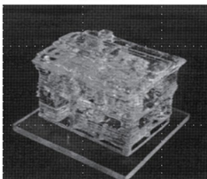
The first model, a house, fabricated by the 3D printer
