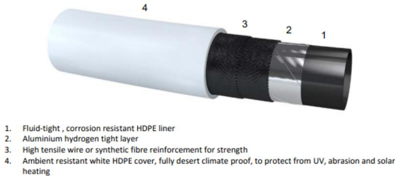
Figure 3.18: Solforce Hydrogen Pipeline (HYGRO, 2021)
