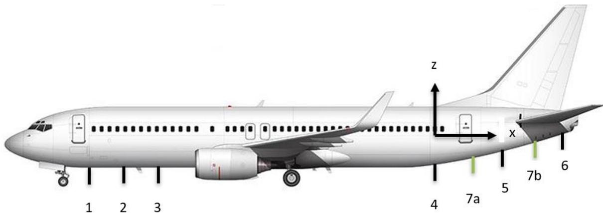
Figure 6.1 Investigated Antenna placement locations for the multiband antenna system
