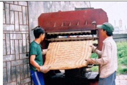
Mats are pressed together under high temperature and pressure to form roofing sheets
