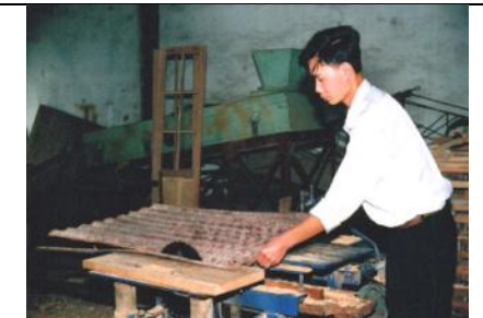
Sheets are trimmed to shape and may then be painted
