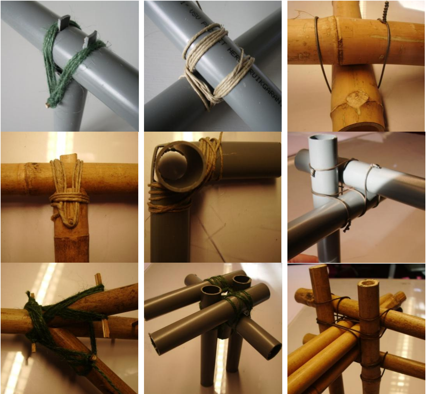
Fig. 4.9 Different ways of jointing with rope and steel wire
