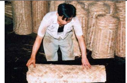
Mats are soaked in adhesive resin
