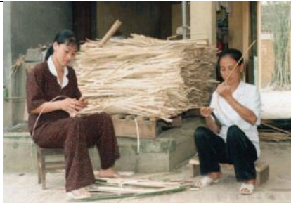
Bamboos are split into thin slivers
