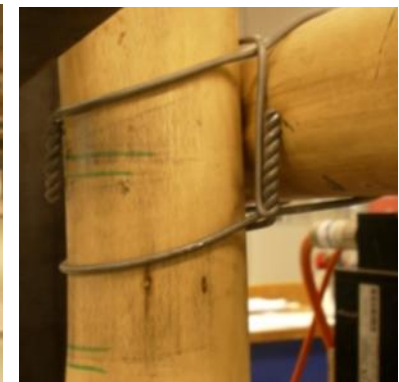
Fig. 6.6 Bamboo joint with extra metal wire after the pressure test
