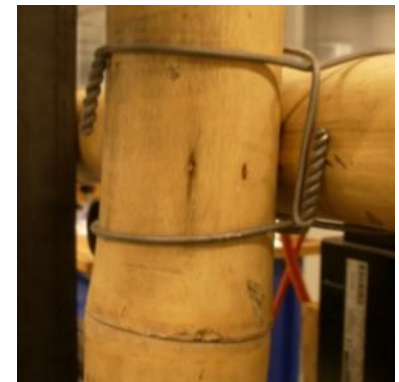
Fig. 6.5 Bamboo joint with extra metal wire
