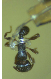
Figure 40: Humped structure holding a ant [44].
