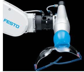
Figure 33: Gripper based on chameleon's tongue [41].
