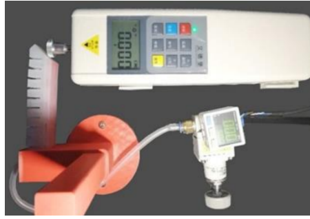
Figure 65: Measuring force with sensor [67].
