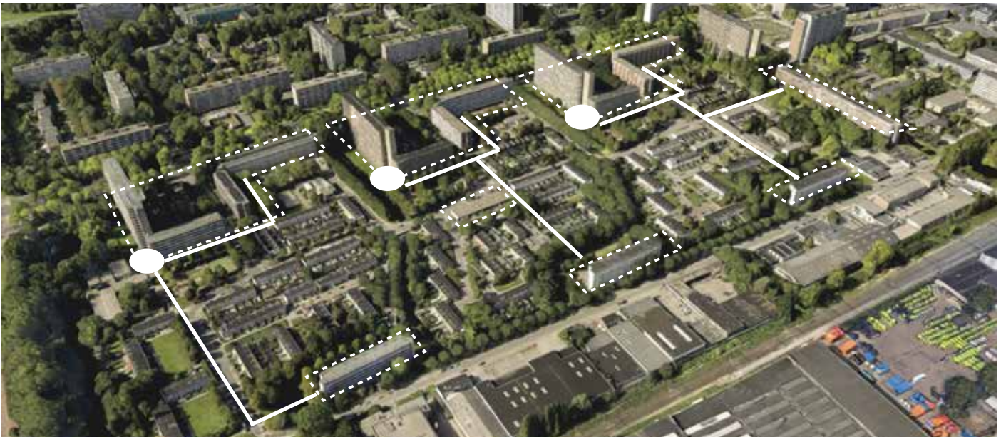
Figure 7.9. The existing inactive heat network in Voorhof-Oost (based on: Schild, et al. 2017).
