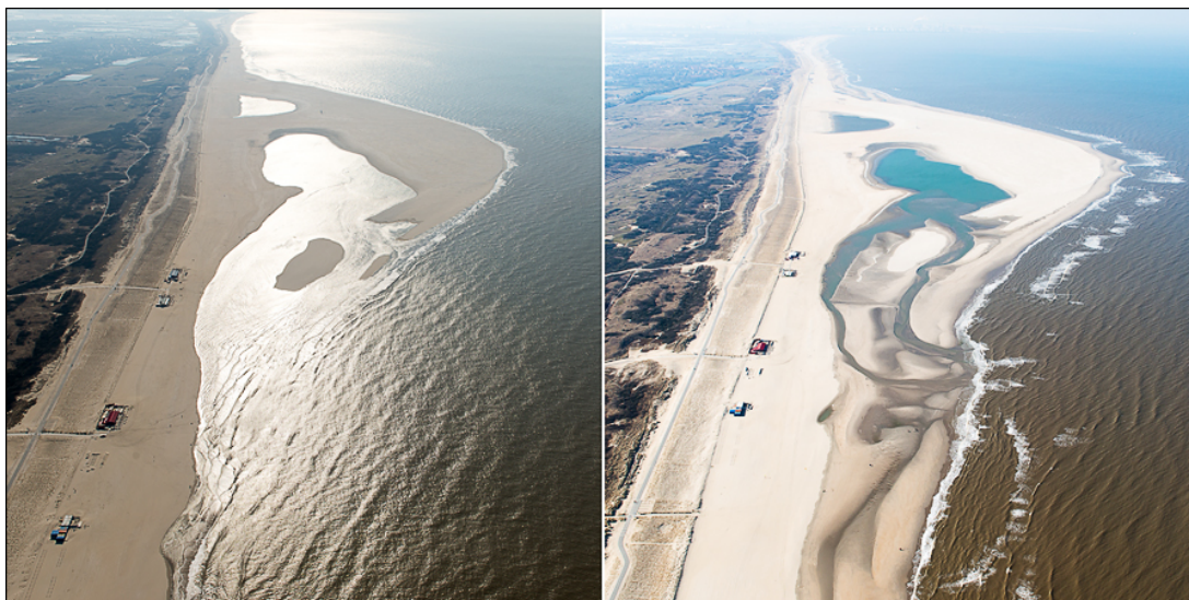
Figure 5 Southward looking aerial photograph of the Sand Engine at high water ( left ) and at low water ( right ) (spring 2013). Pictures courtesy of Rijkswaterstaat/Joop van Houdt.
