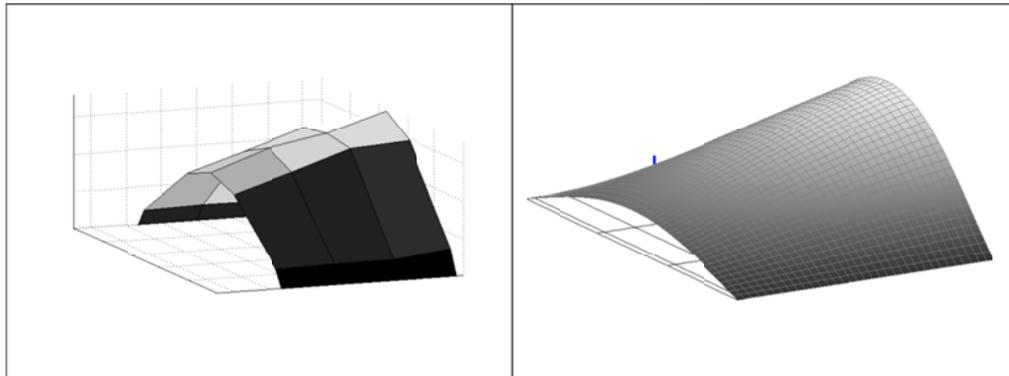
**Fig. 3** First order bending frequency for SSI (left) and FEM (right)
