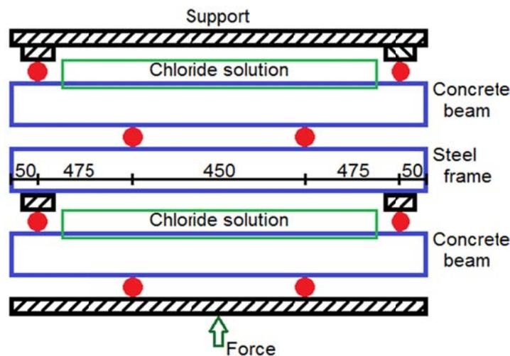
Fig. 5 Draft of the load setup
