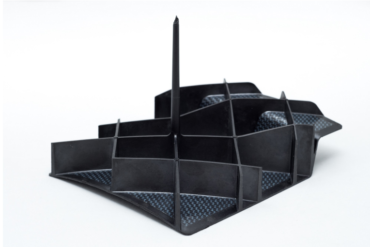
Figure 5.34: Overmolded grid demonstrator made by TPRC. (Courtesy of JEC composites magazine)
