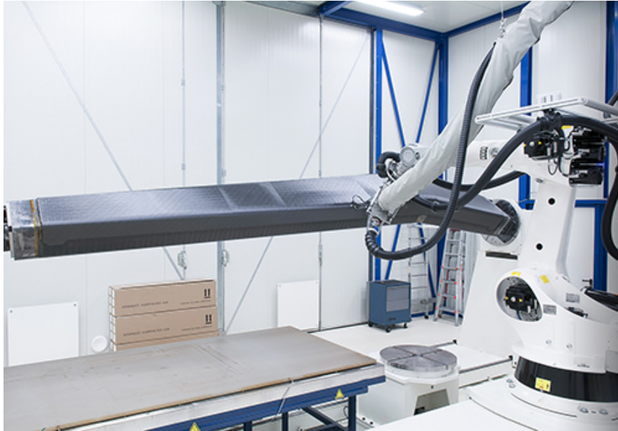
Figure 2.9: AFP of C/PEKK wing pylon spar using laser tacking at the NLR. (Courtesy of the NLR)
