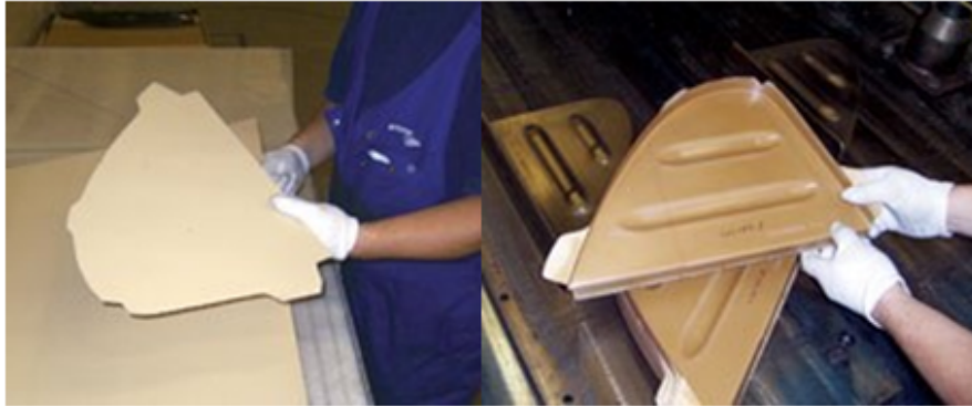
Figure 2.5: Images of A380 J-nose LE rib blank (Left) and press-formed rib (Right). (Courtesy of Composites World magazine)
