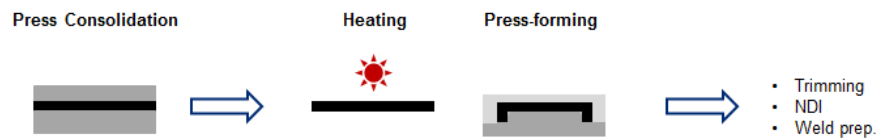
Figure 2.6: Process flow of OoA press-forming.
