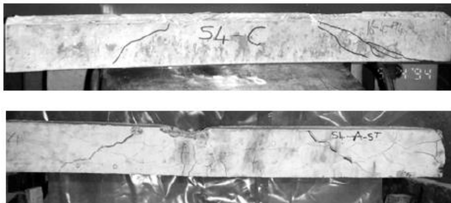
Figure 15 Failure mode for Beam S4-C (top, shear) and S4-A (bottom, bending) (Ahmed, Burley, & Rigden, 1998)
