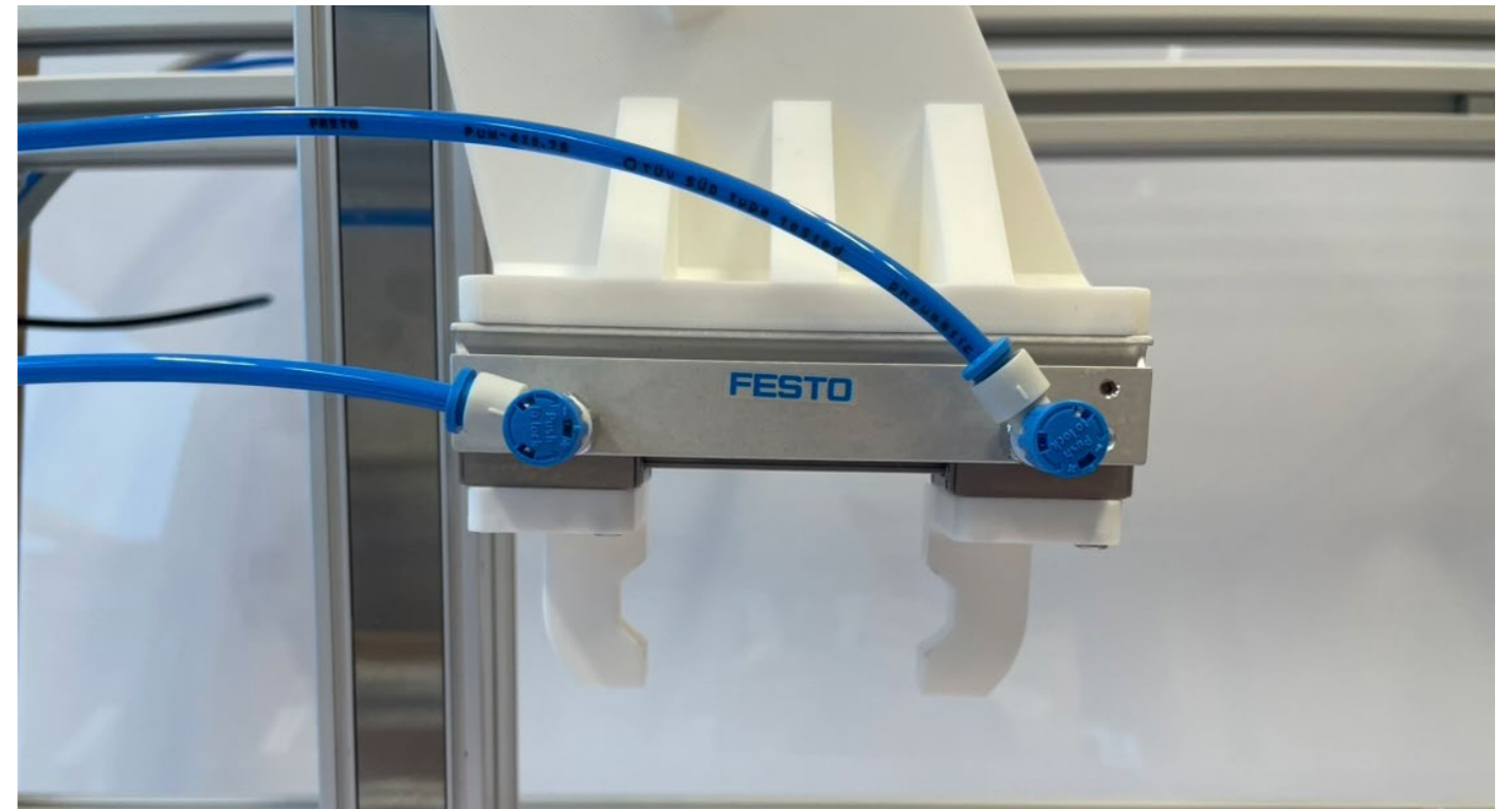
Figure 35 B: Mechanism that holds syringe
