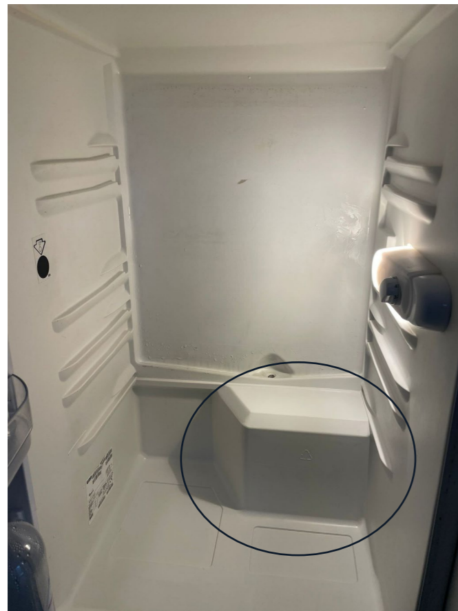
Figure 48: Dedicated volume for the compressor
