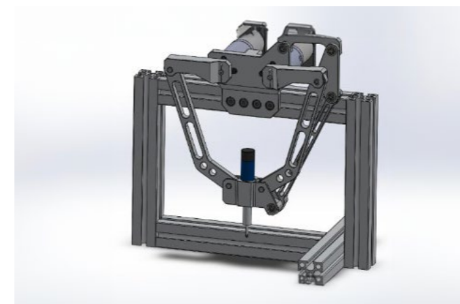
Figure 45: 2D Delta robot Structural Design (Yang et al., 2017)
