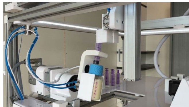
Figure 16: Custom-designed blue connector cap
