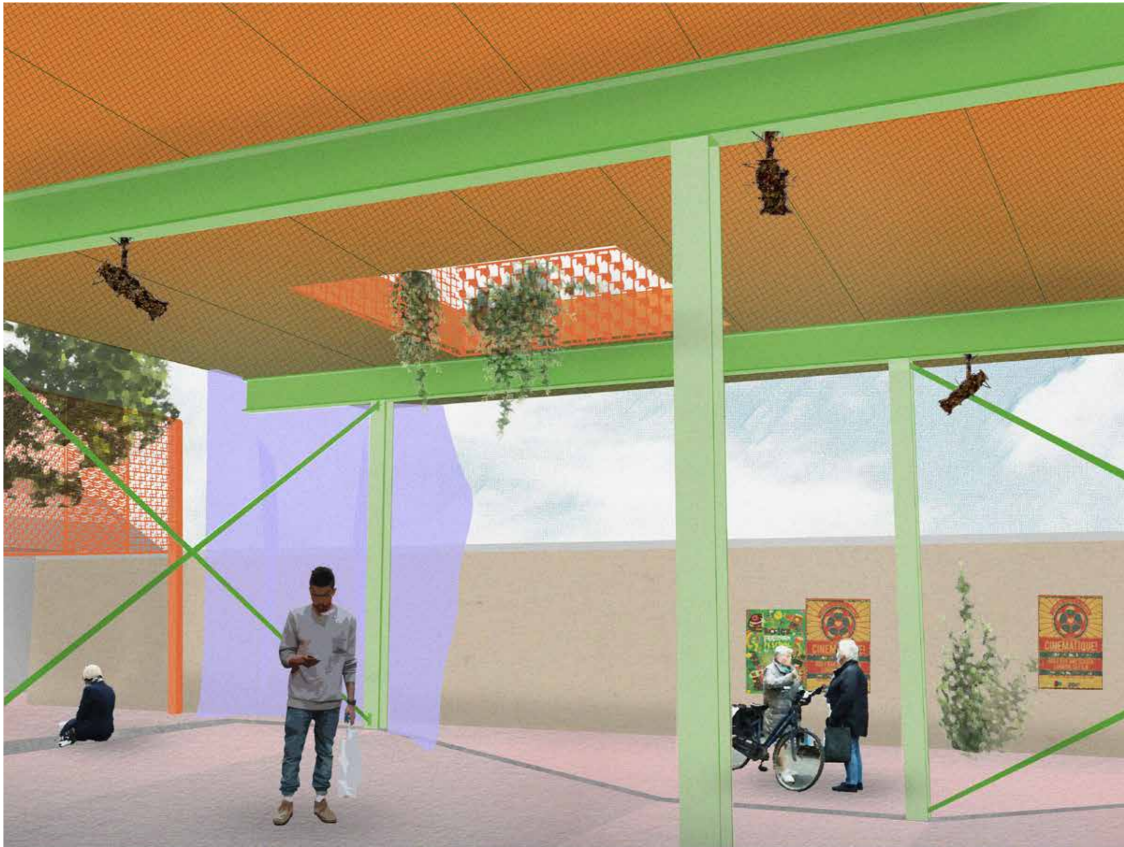
Reused steel, fence, contour plates. Curtain hanging from the ceiling
