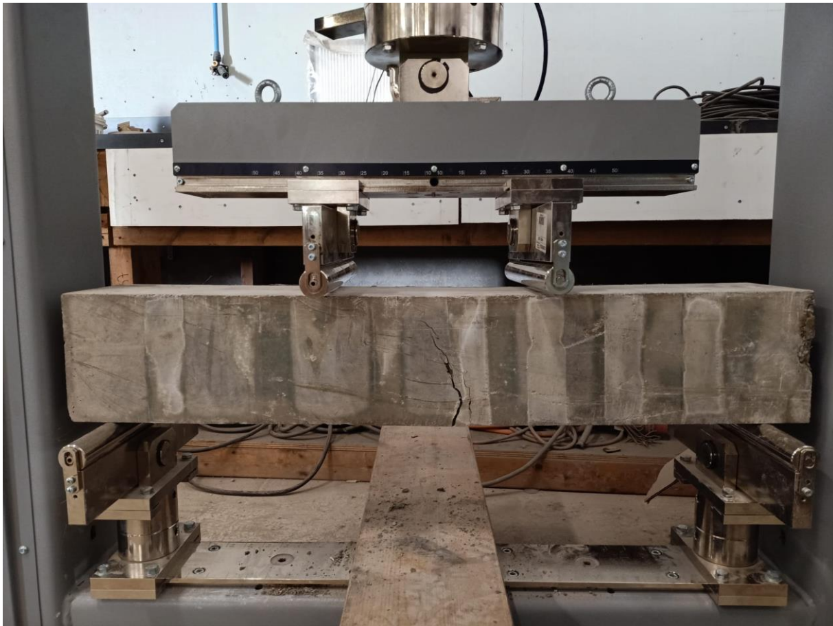
Figure 6.8: 4 point bending test on beam l = 850 mm (30 kg/m 3 Minibars)
