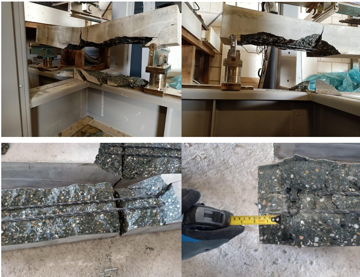
Figures 6.4: Visualisation of concrete spalling off due to anchorage failure
