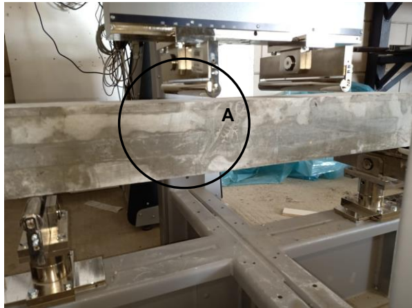
Figure 6.3: Results of 4 point bending test with possible shear failure + detail A (turned out to be anchorage failure)
