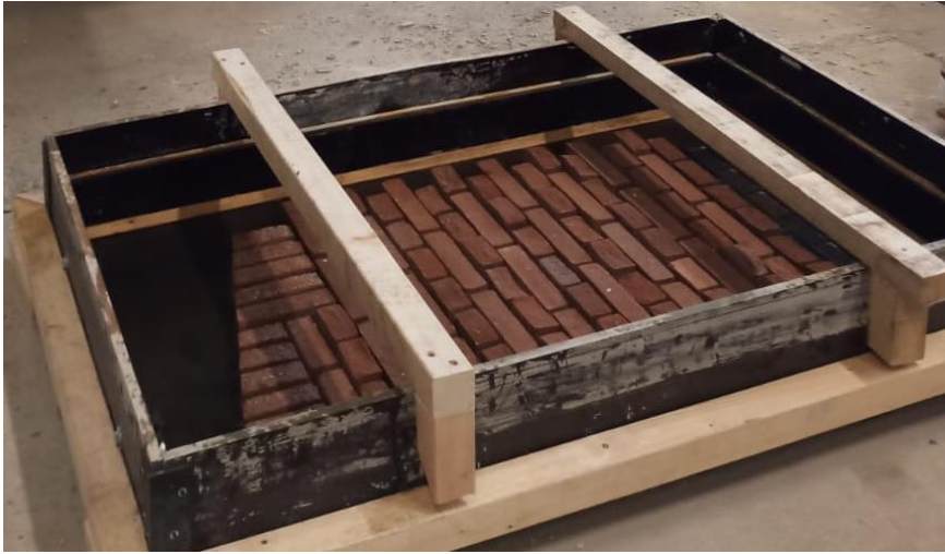
Figure 5.3: The mould with bricks laid into the pattern
