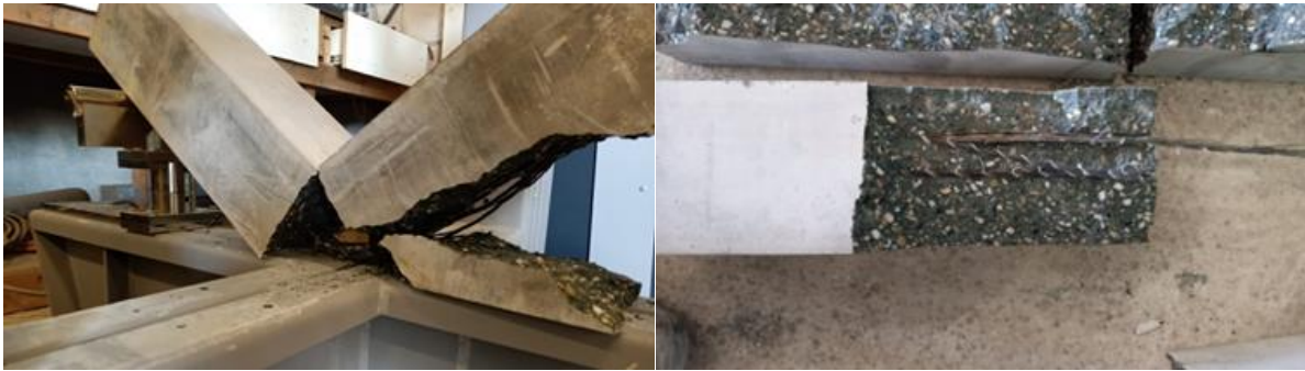
Figure 6.5: Brittle failure of the basbars
