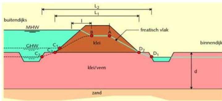
Figure 45 Illustration governing method for schematizing the phreatic surface in a flood defence (TAW, 2004)
