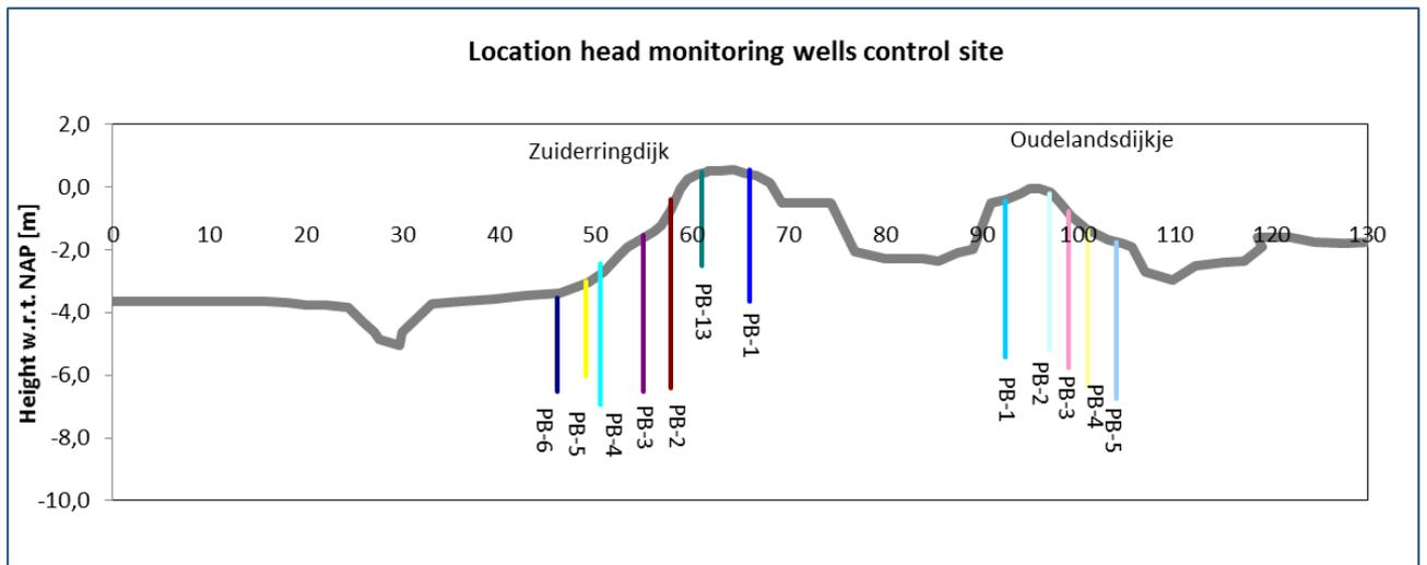
Figure 94 Location head monitoring wells control site
