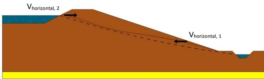
Figure 73 Illustration horizontal travel speed phreatic surface under influence of precipitation
