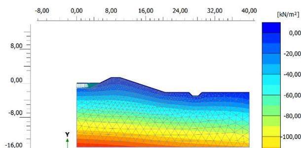
Figure 46 Pore pressures in  $\text{kN/m}^3$  in a fully saturated dike after an extreme precipitation event
