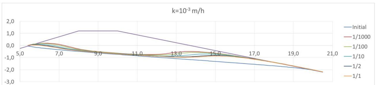
Figure 79 Rise phreatic surface in sand  $k=2,8 \cdot 10^{-7}$  m/s for different return periods
