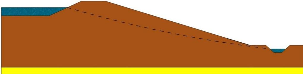
*Figure 5 Schematization ground water table inside regional flood defence*
