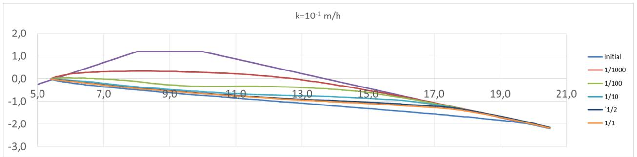
Figure 89 Rise phreatic surface clay  $k=2,8 \cdot 10^{-5}$  m/s for different return periods
