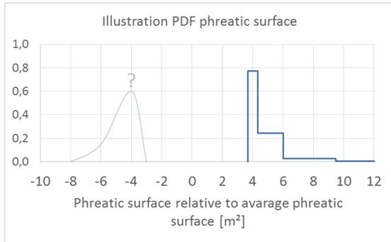
Figure 76 Illustration probability density phreatic surface according to the method developed in this thesis; the shape of the probability density of the low phreatic surface is not studied and randomly chosen.
