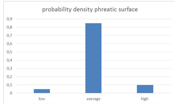
Figure 77 Probability density phreatic surface according to the original method (Lendering, Jonkman, & Kok, 2015)
