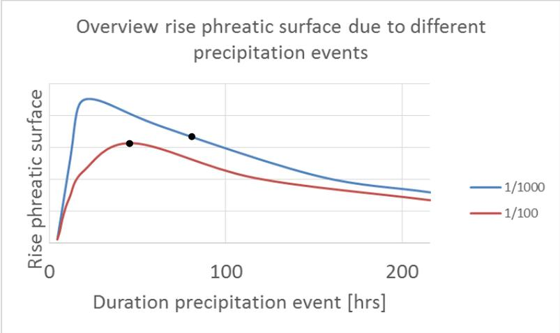
Figure 55 Rise phreatic surface (in a dike with an arbitrary set of soil parameters) due to precipitation events with two different return periods
