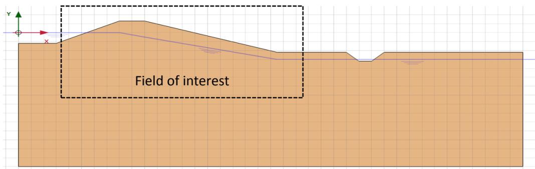
Figure 33 Cross section dike used in FEM
