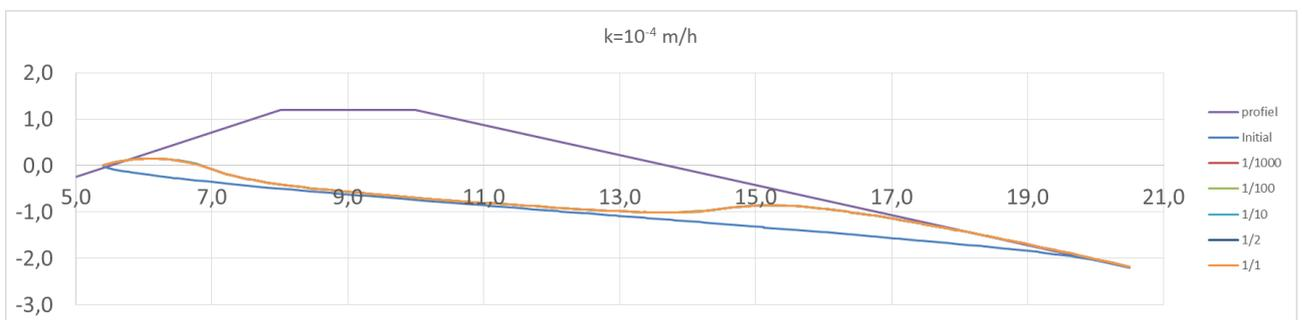
Figure 86 Rise phreatic surface clay  $k=2,8 \cdot 10^{-8}$  m/s for different return periods
