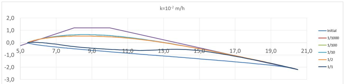
Figure 88 Rise phreatic surface clay  $k=2,8 \cdot 10^{-6}$  m/s for different return periods
