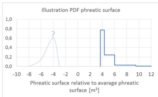
Figure 63 Illustration probability density distribution of the phreatic surface
