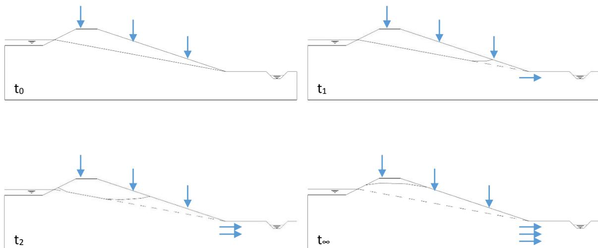
Figure 18 Illustration process of the effect of precipitation in the phreatic surface over time until an equilibrium is reached
