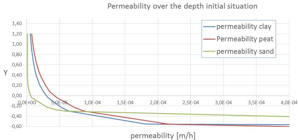
Figure 37 Unsaturated permeability in the top layer of the dike in the initial situation
