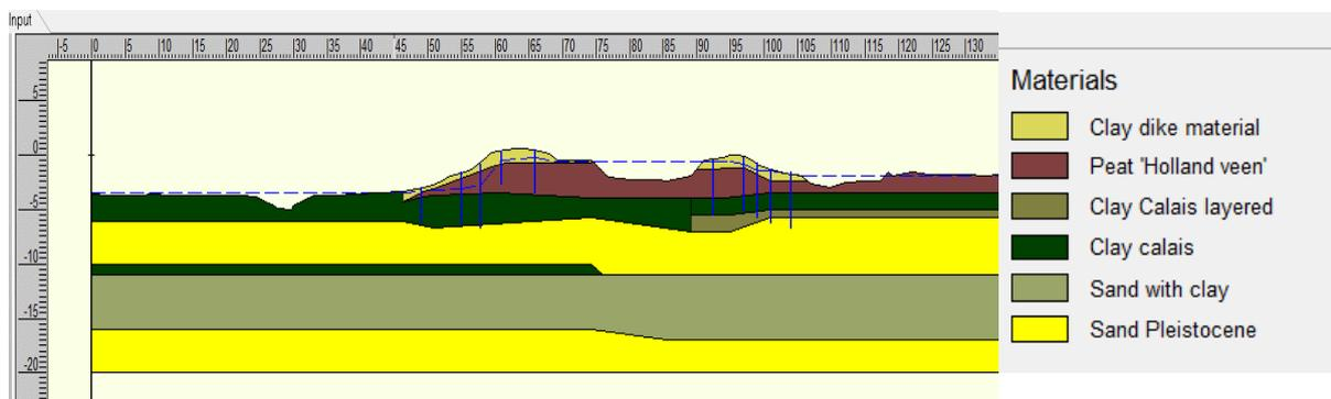
Figure 91 Schematization test site
