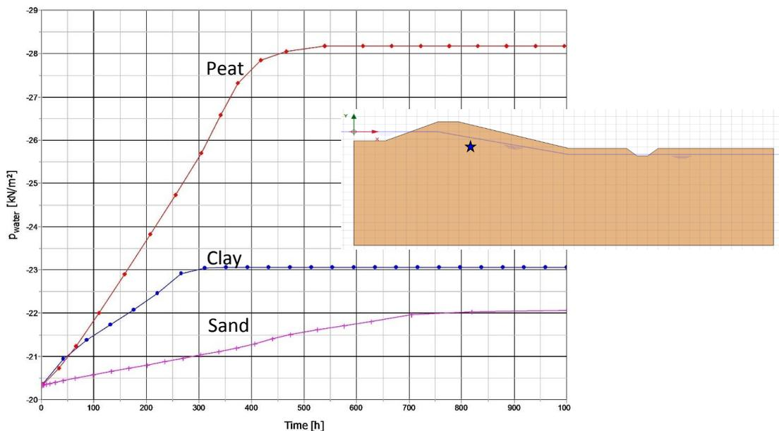
Figure 38 Development pore pressures of clay, peat and sand; precipitation intensity of 0,25mm/h
