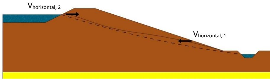
Figure 78 Illustration horizontal travel speed phreatic surface under influence of precipitation
