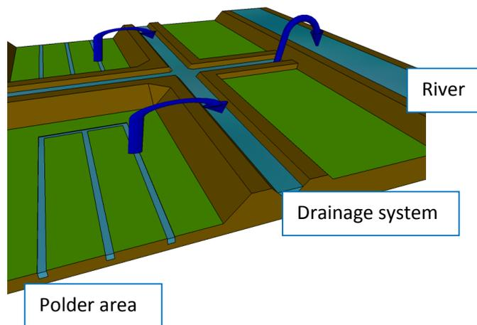
Figure 2 Illustration polder drainage system
