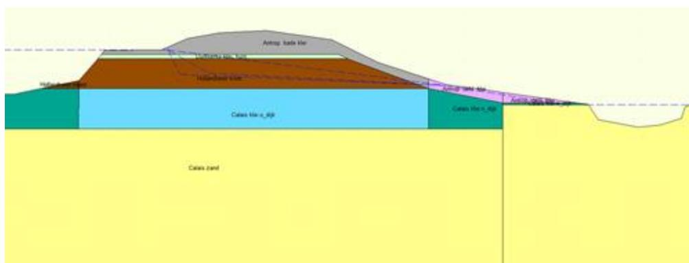
Figure 70 Illustration schematization phreatic surface section 17; original method (Lendering, Jonkman, & Kok, 2015)
