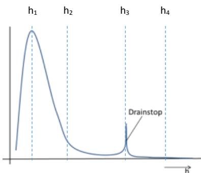
Figure 64 Probability density function water level in drainage canal (Lendering, Jonkman, & Kok. 2015)
