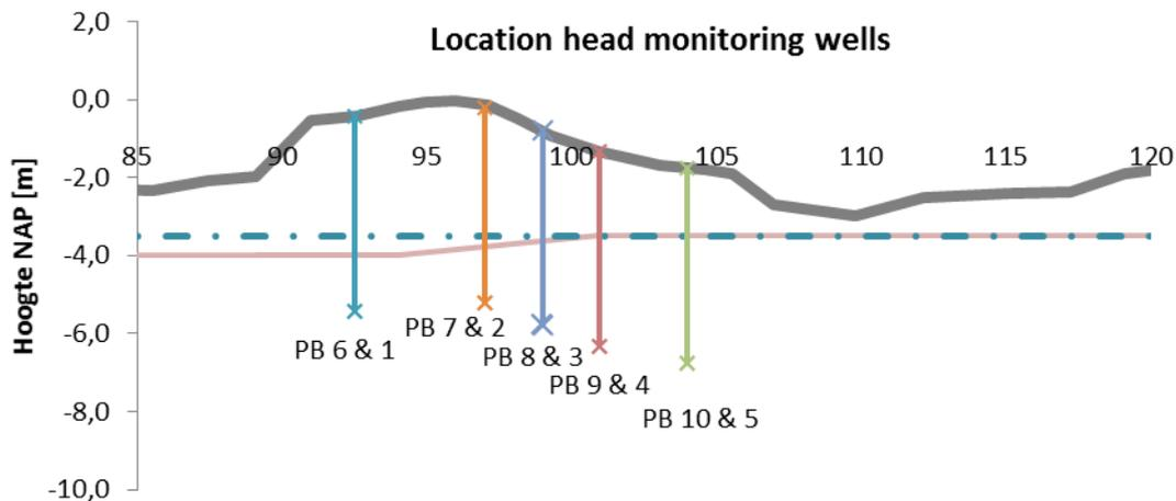
Figure 30 cross section and head monitoring wells 'Oudelandsdijkje'
