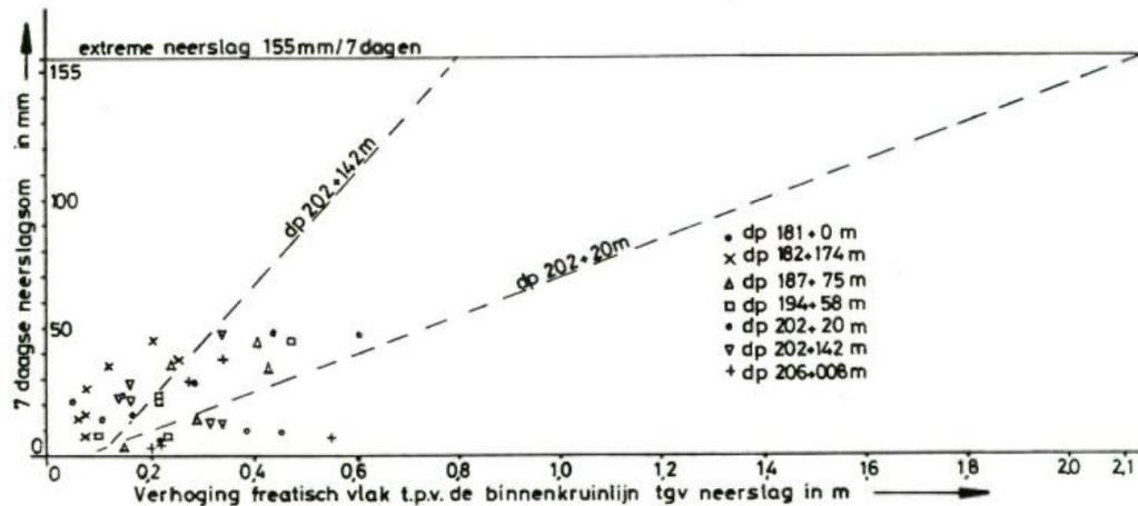
Figure 19 Relation precipitation-increase phreatic surface at the location of the inner crest line (GeoDelft, 1990)
