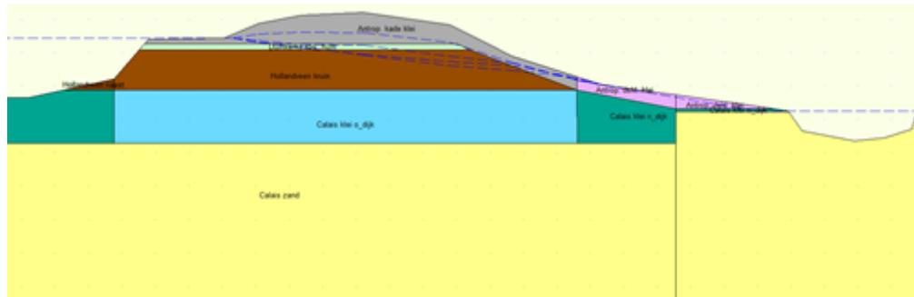
Figure 71 Illustration schematization phreatic surface section 17; new method
