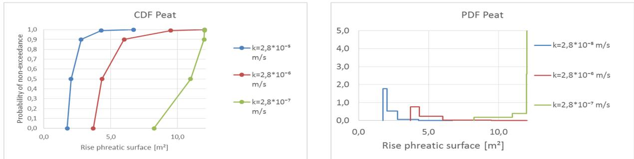
Figure 60 Cumulative density function and probability density function; peat
