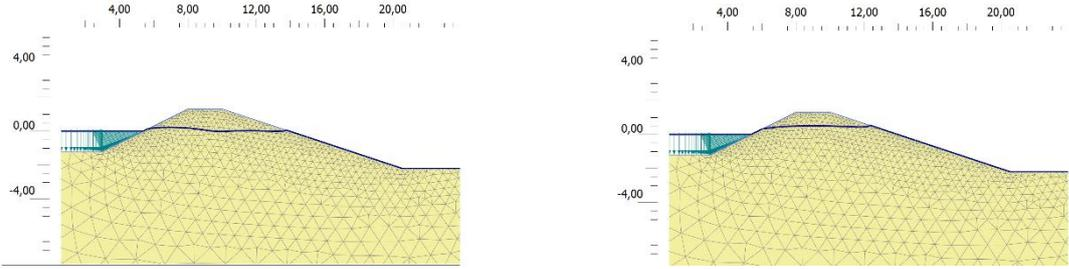
Figure 44 Illustration development phreatic surface at t=300 (left) and t>500 (right)
