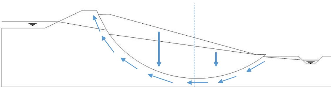
Figure 10 Schematization mechanical aspects macro instability
