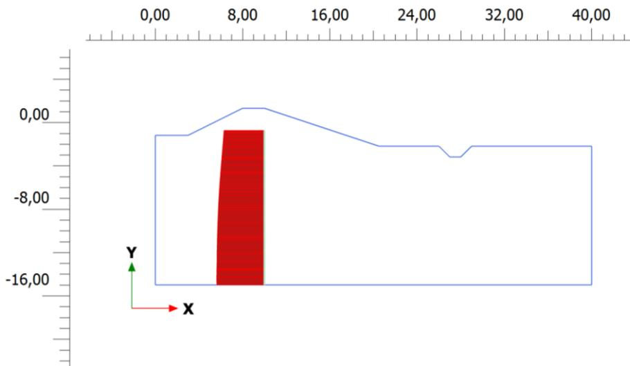
Figure 40 Ground water head over the depth in neutral situation: Maximum: -0,97m and minimum -1,06m
