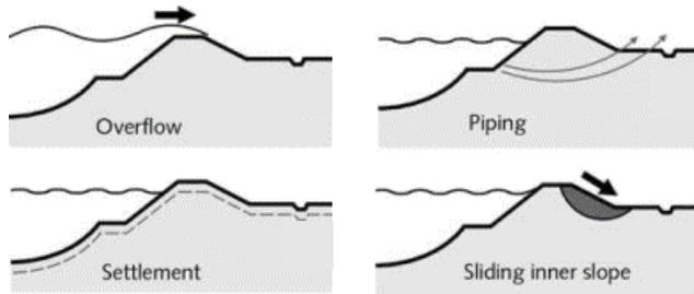
Figure 9 Dominant failure mechanisms regional flood defence system (TAW, 2001)
