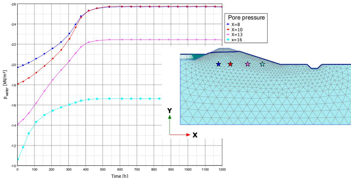
Figure 42 Pore pressure rise at underneath the crest and the slope of a dike of peat for an infinite event of 0,25mm/h (left) Phreatic surface at  $t=\infty$  for a precipitation event of 0,25mm/h on a peat dike (right)
