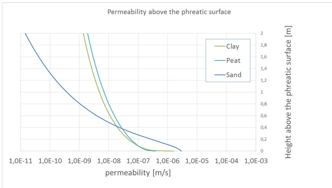
Figure 34 Permeability of the materials sand, clay and peat as used in the computation
