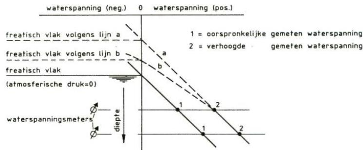
Figure 20 Pore pressure over the depth (GeoDelft, 1990)
