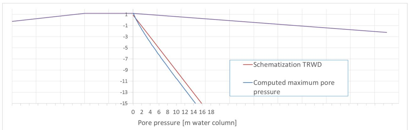
Figure 47 Comparison between the maximum schematized pore pressures according to the TRWD and the maximum computed pore pressures
