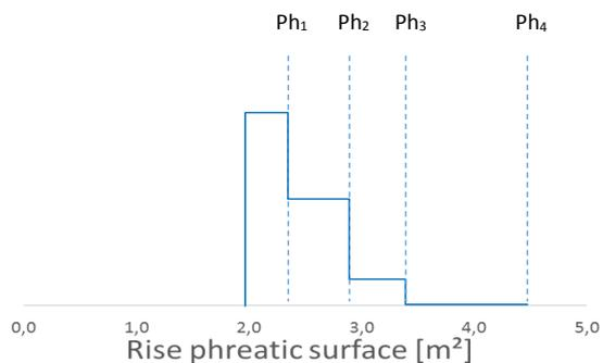
Figure 65 Probability density function rise phreatic surface due to precipitation
