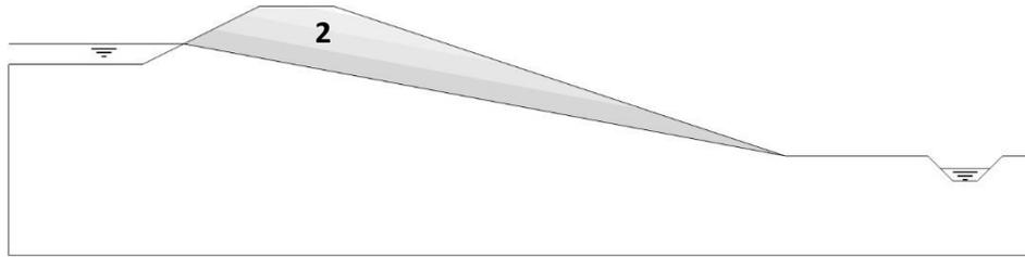
Figure 16 Illustration unsaturated zone above the phreatic surface
