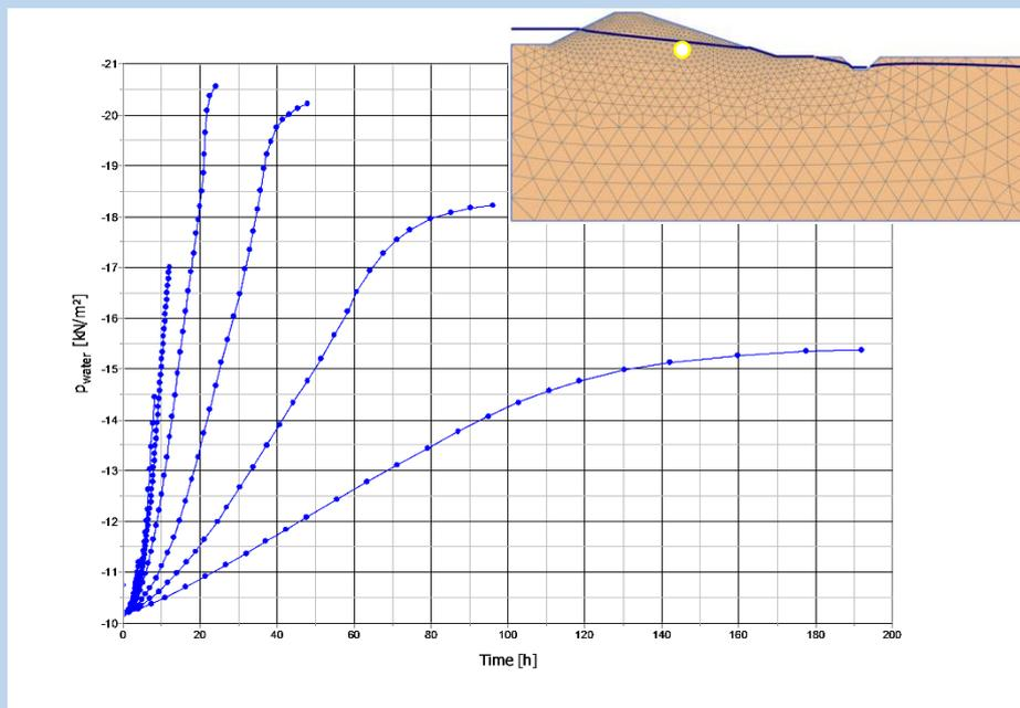
Figure 52 Pore pressure rise due to multiple events with a return period of 100 years
