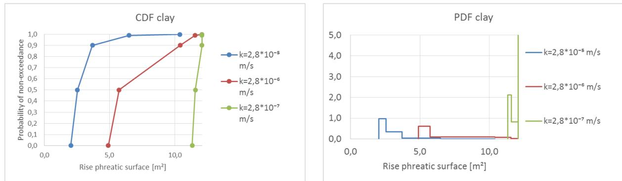
Figure 61 Cumulative density function and probability density function; clay
