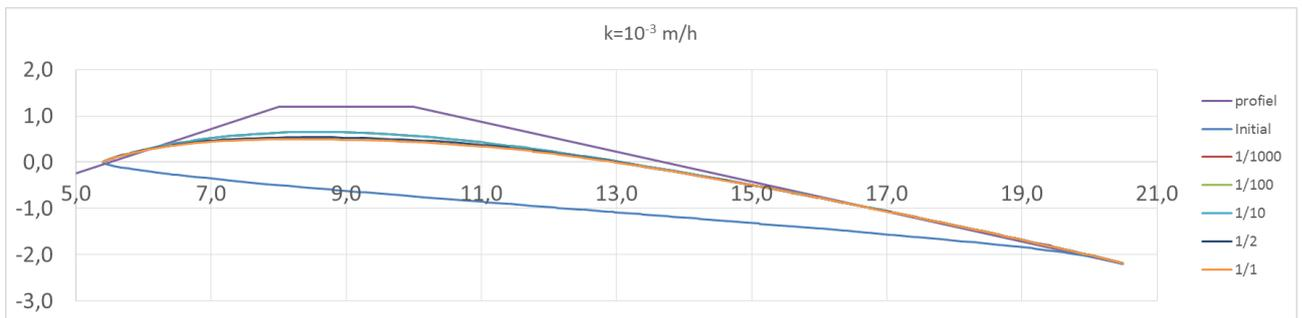
Figure 87 Rise phreatic surface  $k=2,8 \cdot 10^{-7}$  m/s for different return periods
