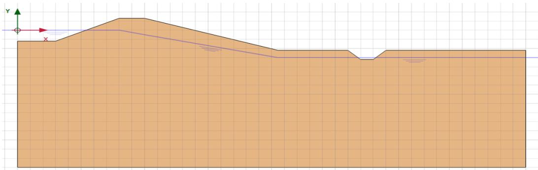
Figure 58 Schematization of a regional flood defence for the computation of the phreatic surface
