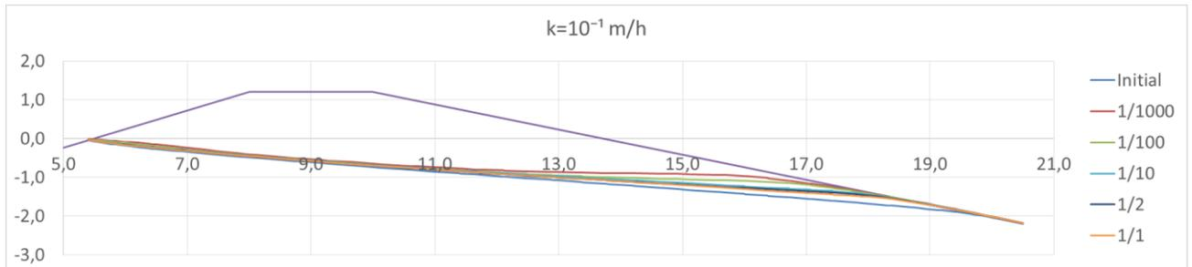
Figure 81 Rise phreatic surface in sand  $k=2,8 \cdot 10^{-5}$  m/s for different return periods
