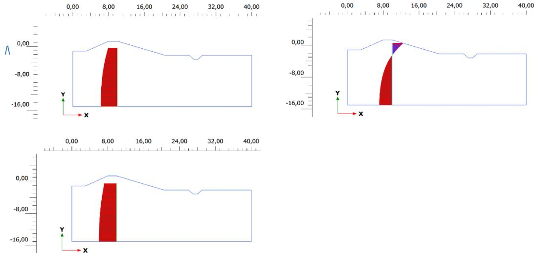
Figure 41 Equilibrium ground water head for clay (top left), peat (top right) and sand (bottom) with a precipitation intensity of 0,25 mm/h at the inner crest line ( $x=10$ )
