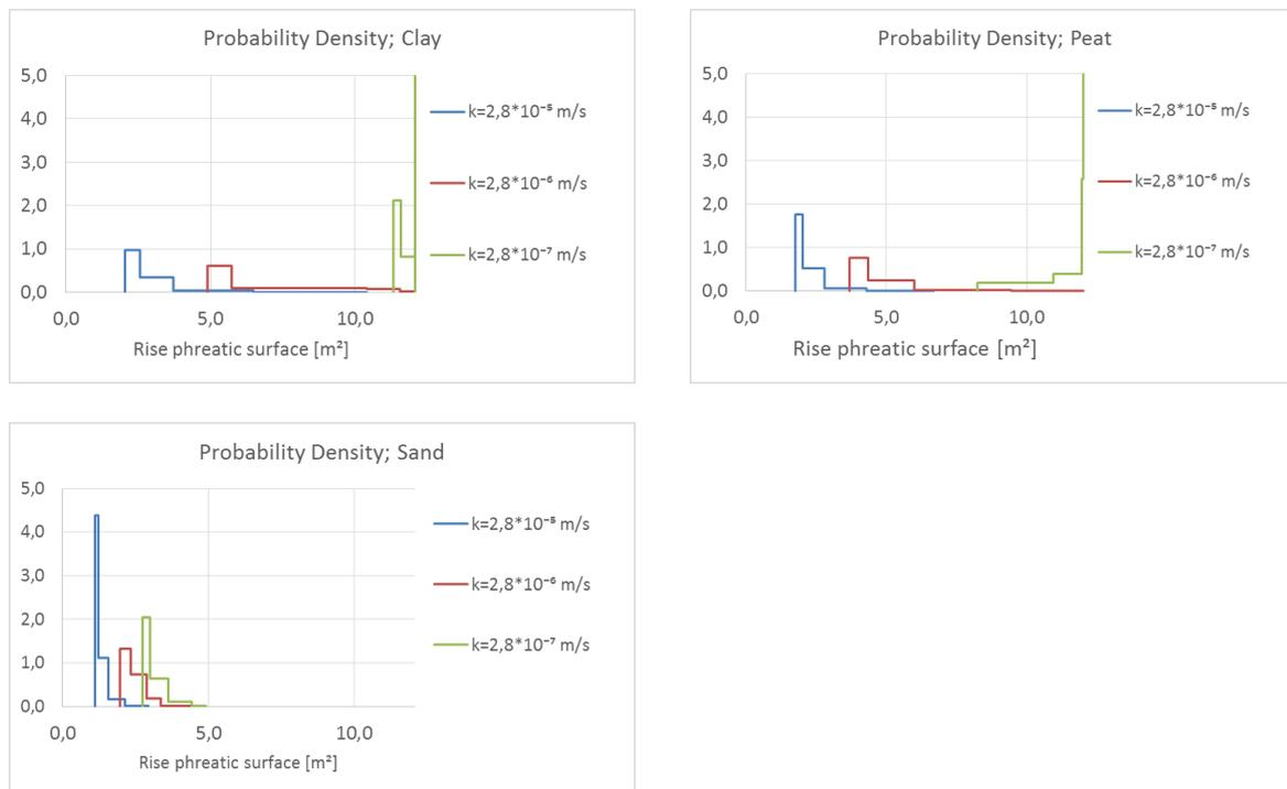
Figure 1 Probability density functions for a dike of clay, peat and sand for different degrees of permeability
