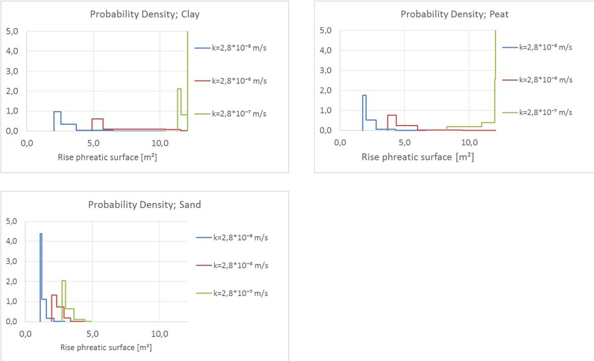
Figure 74 Probability density functions for a dike of clay, peat and sand for different degrees of permeability
