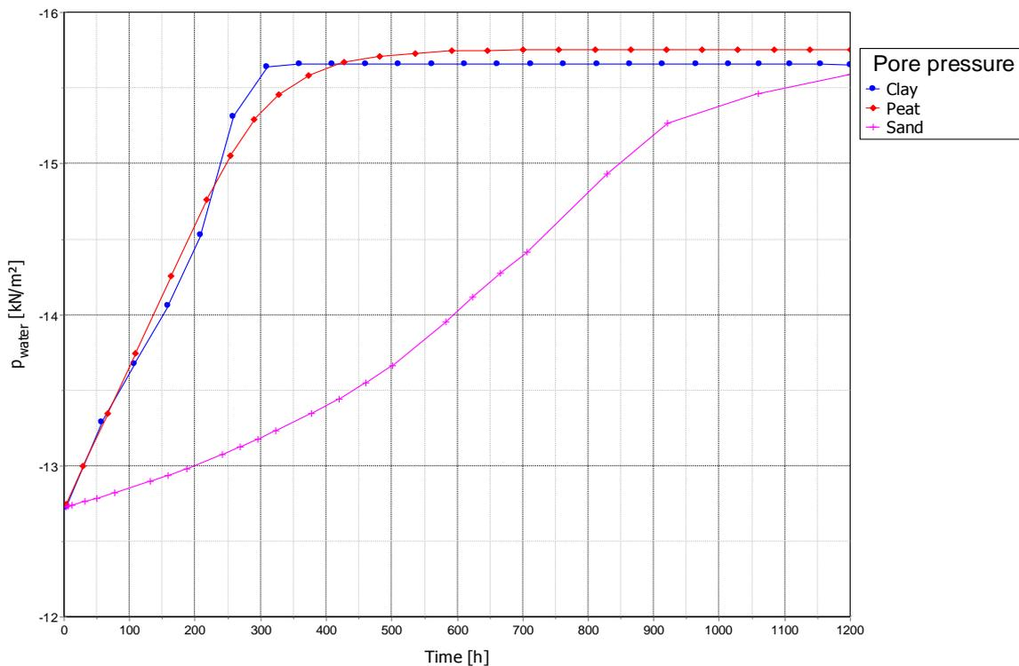
Figure 39 Pore pressure development for clay, peat and sand with a permeability of  $1,4 \cdot 10^{-6}$  m/s for an infinite precipitation event of 0,25mm/h
