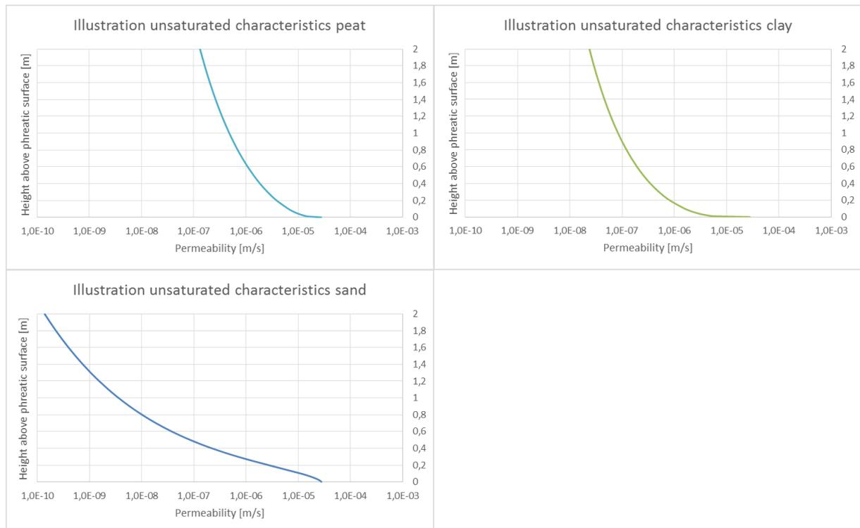
Figure 17 Illustration unsaturated characteristics peat (top left) clay (top right) and sand (bottom)
