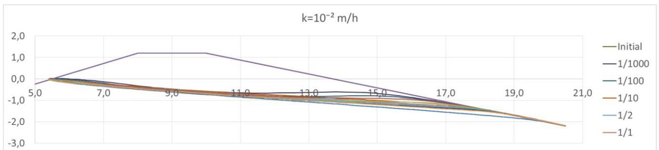
Figure 80 Rise phreatic surface in sand  $k=2,8 \cdot 10^{-6}$  m/s for different return periods
