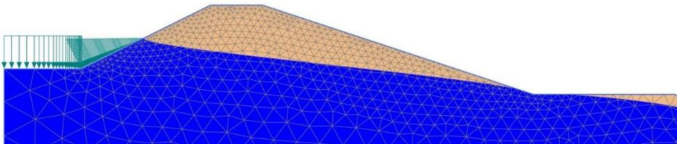
Figure 48 Illustration initial/neutral phreatic surface; starting point for each computation
