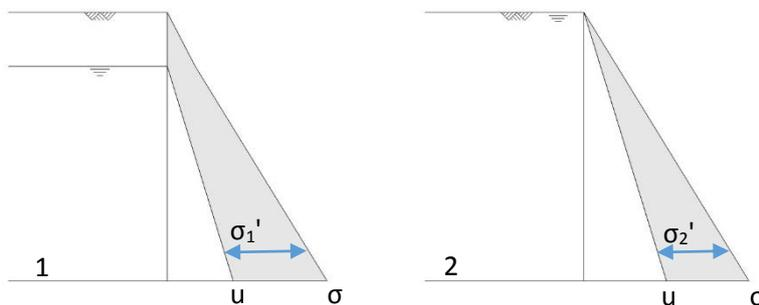
Figure 12 Illustration of the effect of the pore pressure on the effective stress;  $\sigma_1' > \sigma_2'$  due to the increased groundwater level in situation 2.
