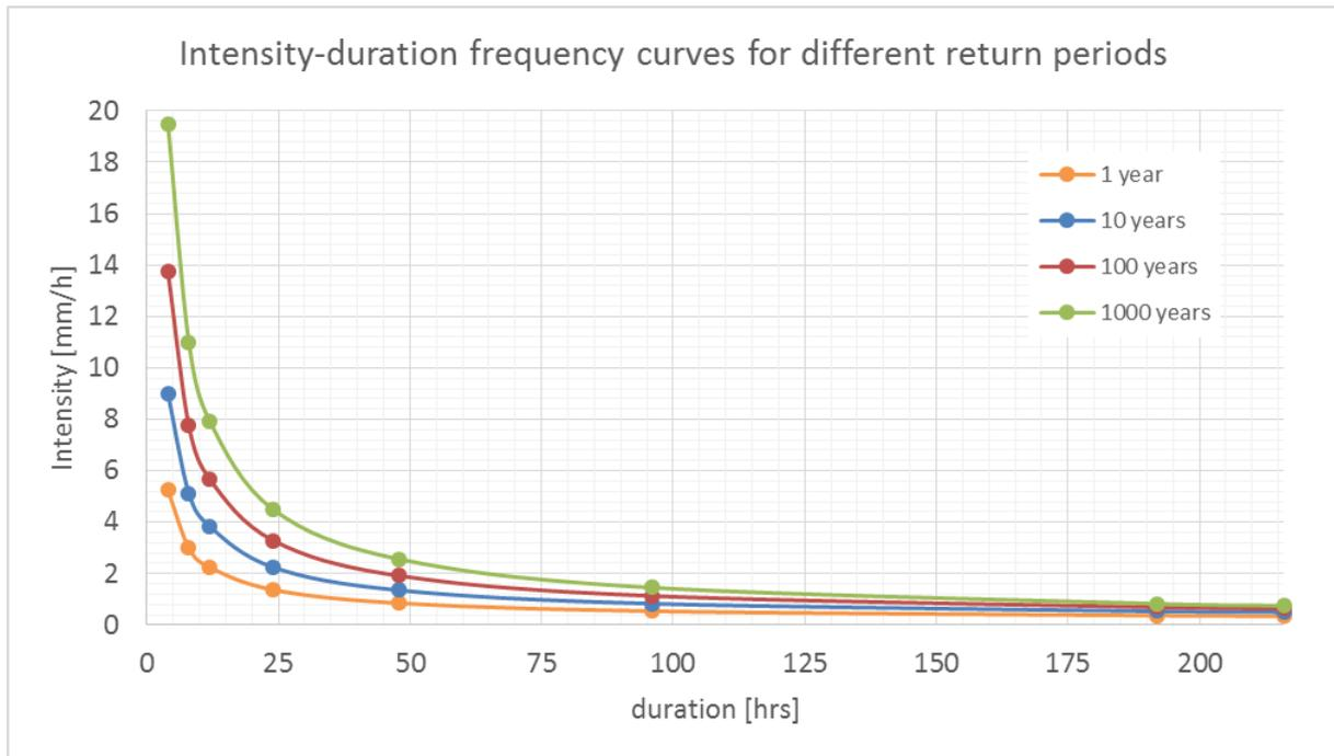
Figure 51 Intensity duration frequency curve for different return periods in de Bilt
