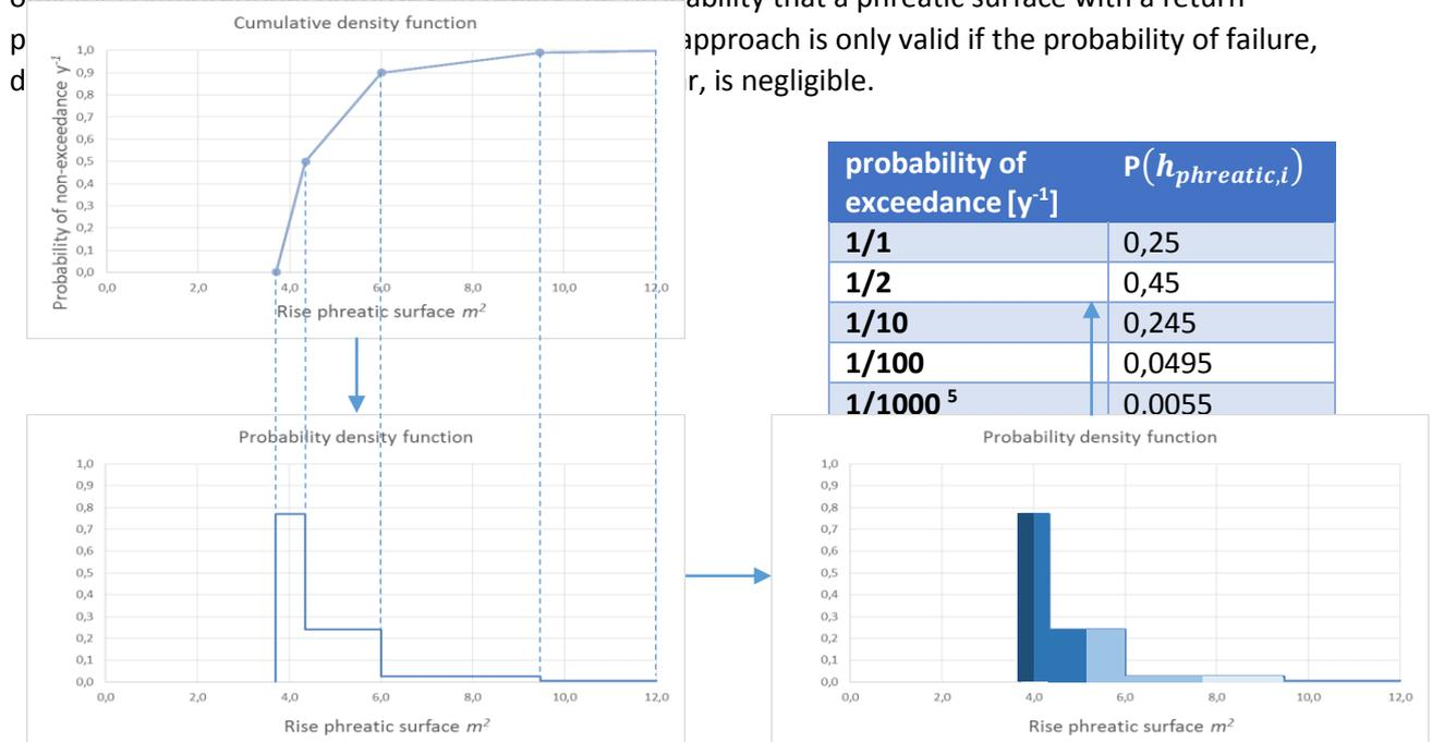
Figure 57 Integration of the PDF in order to compute the probability mass ( $P(h_{\text{phreatic},i})$ ) per computed level of the phreatic surface
