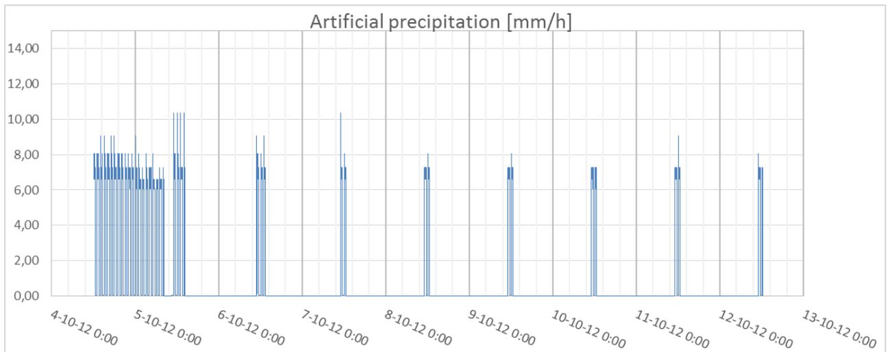
Figure 92 pattern artificial precipitation test Oudelandsdijkje
