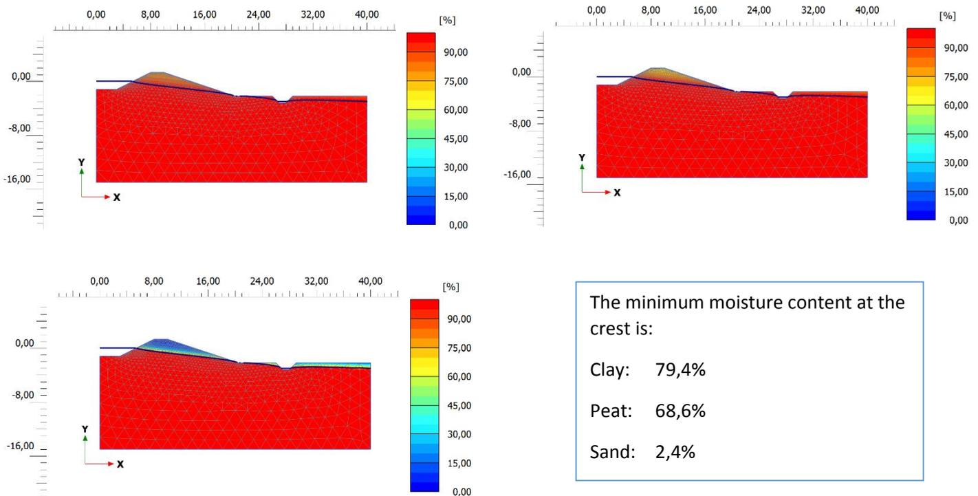
Figure 36 Initial moisture content clay (top left), peat (top right) and sand (bottom left)
