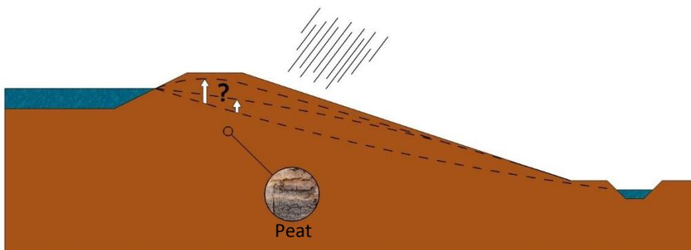
Figure 26 research target Ch. 4 : influence of precipitation on the pore phreatic surface inside a peat dike
