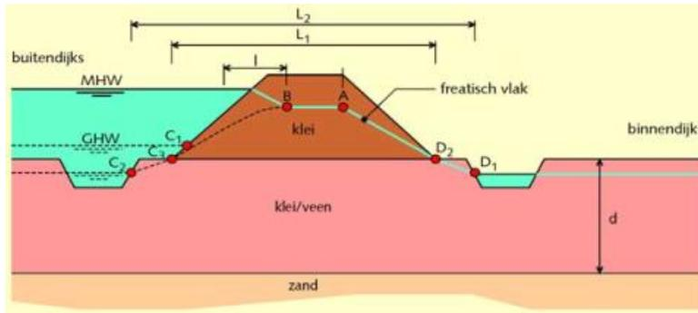
Figure 22 Schematization guideline phreatic surface for a clay dike on a sand base (TAW, 2004)
