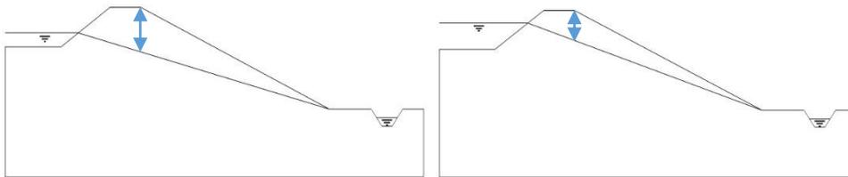
Figure 50 Illustration effect relative crest height on the distance between the phreatic surface and the crest
