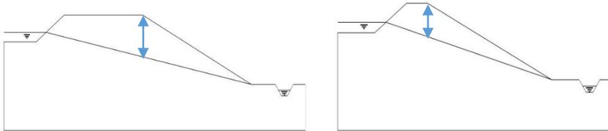
Figure 49 Illustration effect dike width on the distance between the phreatic surface and the crest
