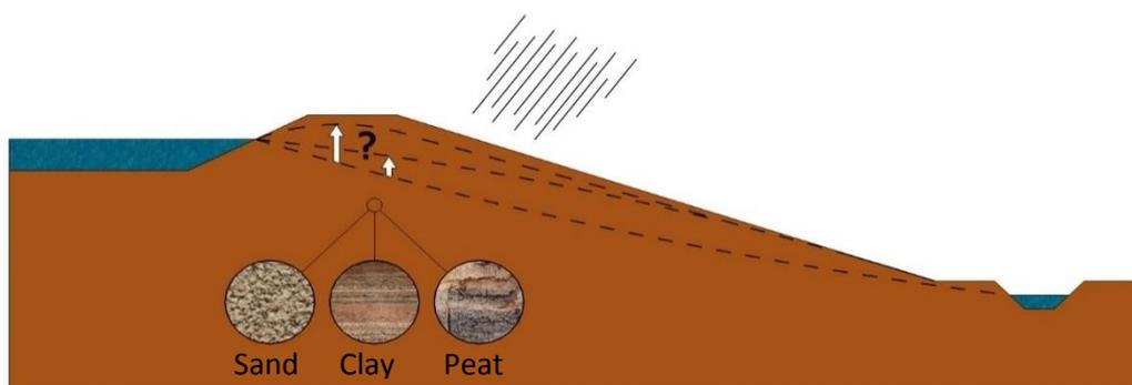
Figure 32 Research goal Chapter 6: general information development pore pressures due to precipitation
