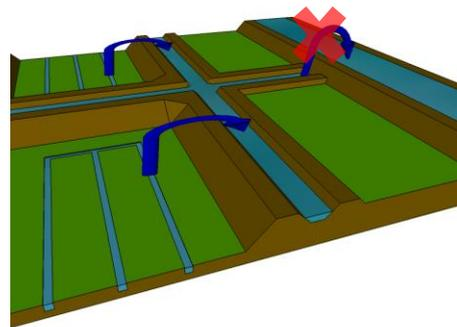
Figure 67 situation 2: pumping capacity to outside water zero due to river flood
