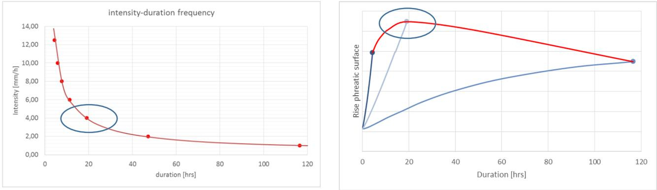
Figure 53 Different combinations of intensity and duration (left) are simulated; the corresponding rise of the phreatic surface is depicted (right). The precipitation event which causes the largest rise of the phreatic surface (blue circle) is called the critical event.
