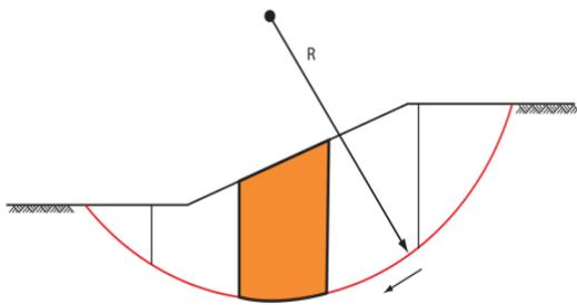
$$F_s = \frac{M_{R;soil} + M_{R;end\ section}}{M_{D;soil} + M_{D;water} + M_{D;load}} \quad (5)$$
