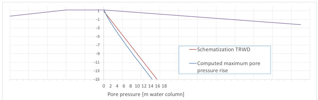
Figure 75 Comparison of the pore pressure, in meters water column, between the TRWD (hydrostatic) and the computation (non-hydrostatic)
