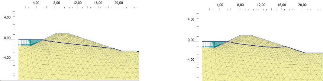
Figure 43 Illustration development phreatic surface at t=0 (left) and t=50 (right)
