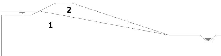
Figure 14 Illustration saturated and unsaturated zones in a dike
