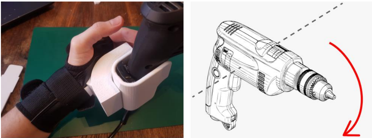
Figure 58A and B. A shows the position of the hand in relation to the drill handle. In this position the drill tends to topple forward, 58B shows the direction more clearly.
