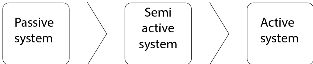
Figure 386: The order in which the basic vibration mitigating technologies should be pursued, with regard to a MVP.
