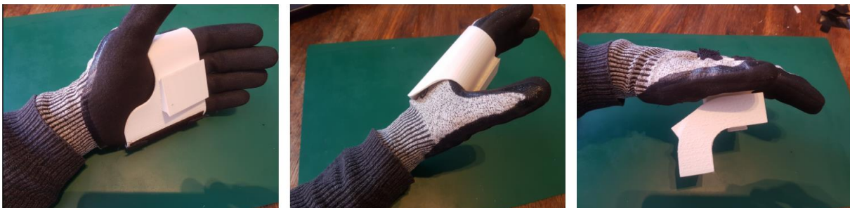
Figure 89A B and C. A shows the palm brace with the connection ledge. B shows the fully enveloping hand brace. C Shows the half palm brace strapped to the hand, with the buffer attached.
