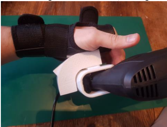
Figure 55A and B. A shows the drill being held on its side. This increases the moment exerted on the brace. 55B shows the direction of this force.
