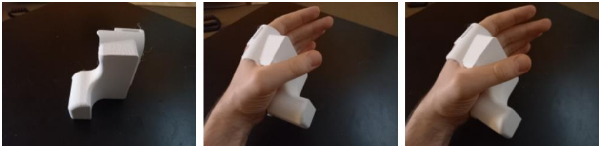
Figure 65A, B and C. The second buffer prototype, with more room for the thumb to move.
