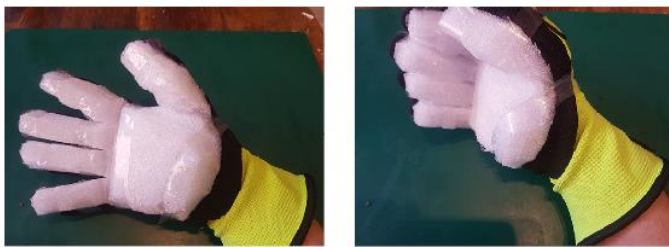
Figure 48A and B, First prototype. Thick padding covering the palm and fingers.
