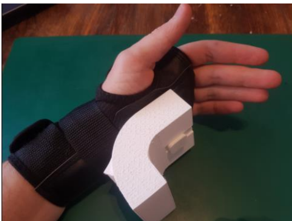
Figure 56A and B. A shows the straight wrist mount, with the buffer attached. 56B: When holding the drill, the fingers can easily reach the controls.
