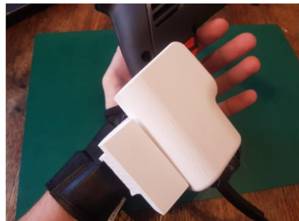
Figure 56A and B. A shows the straight wrist mount, with the buffer attached. 56B: When holding the drill, the fingers can easily reach the controls.
