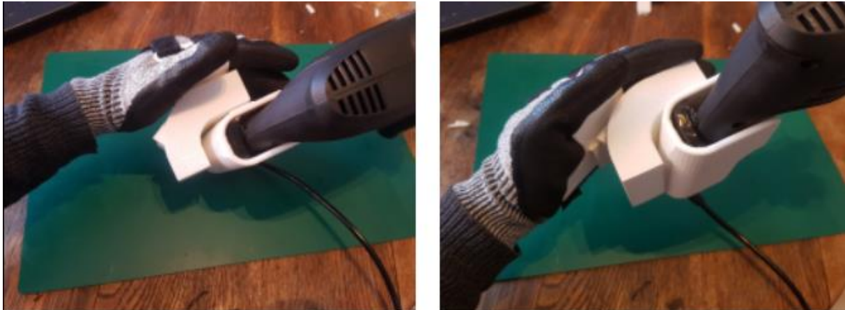
Figure 60A and B Show the palm brace holding the buffer in two positions.
