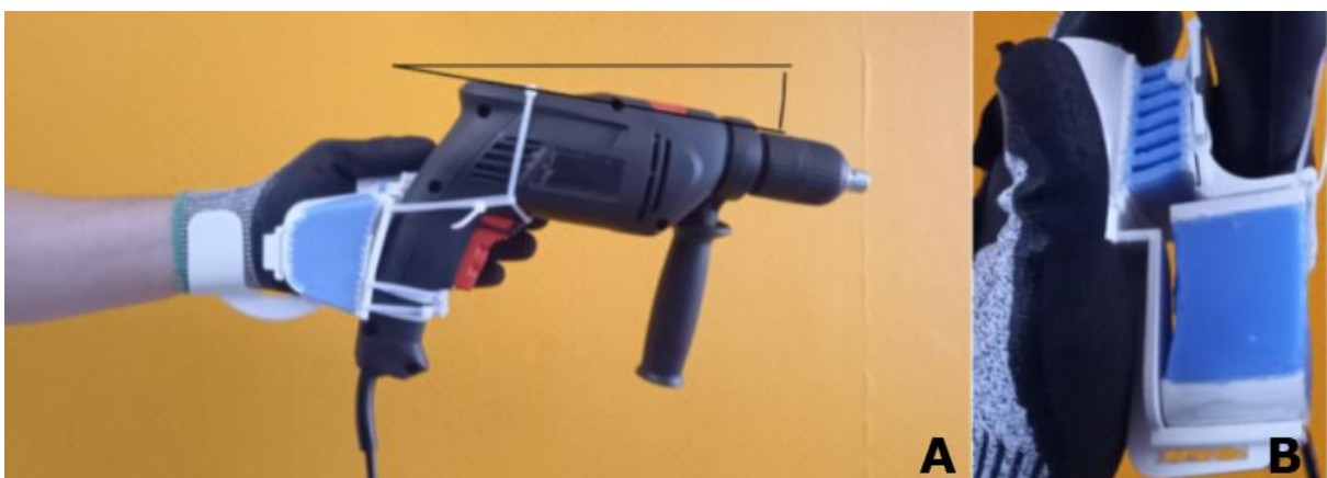
Figure 72A and B. 72A shows that the power tool topples forward significantly. 72B shows in detail how the buffers deform.
