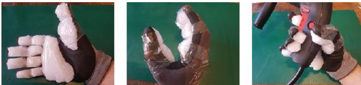
Figure 49A, B and C: Second prototype. Adjusted to the hand with splits to make grasping easier.
