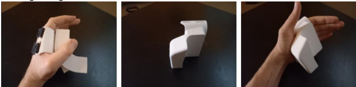
Figure 64A, B and C. A Shows the original place holder buffer, compared with the first buffer prototype shown in B and C.
