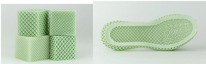
Figure 40 and 41: Lattice structures used in a shoe sole concept.
