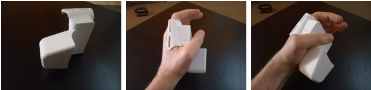
Figure 66 A, B and C. The third buffer prototype, with an extended buffer volume towards the wrist.
