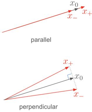
Figure 9: Visualization of the two types of perturbations considered by the authors in their criticality analysis of the kernel.  $x_0$  represents the coincident limit.
