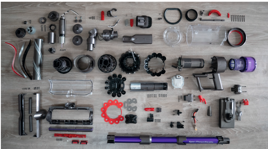
Figure 4.1. The disassembled Dyson V11.
