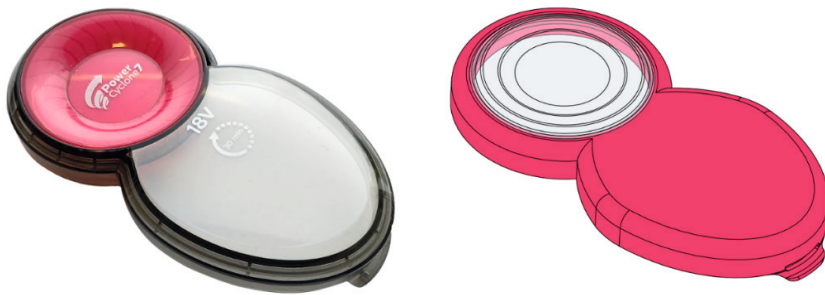
Figure 6.8. The part designs for injection moulding (left) and additive manufacturing (right) are functionally equivalent but not identical. The clear and opaque sides are switched because transparent additive manufacturing materials lack the necessary strength and impact resistance for the lid's main body. Transparent injection-moulding materials do, which is why the main body can be made transparent for better visibility inside the dustbin.
