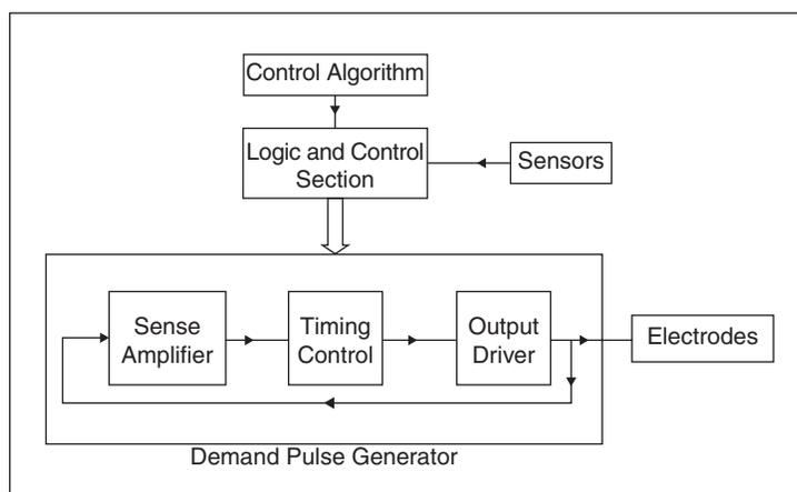
Fig. 9. A block diagram of a rate-responsive pacemaker.
