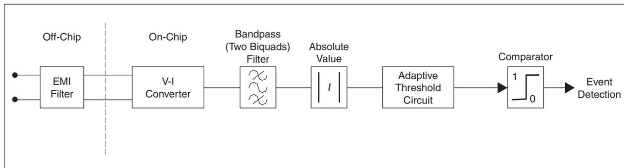
Fig. 10. A block diagram of a sense amplifier.
