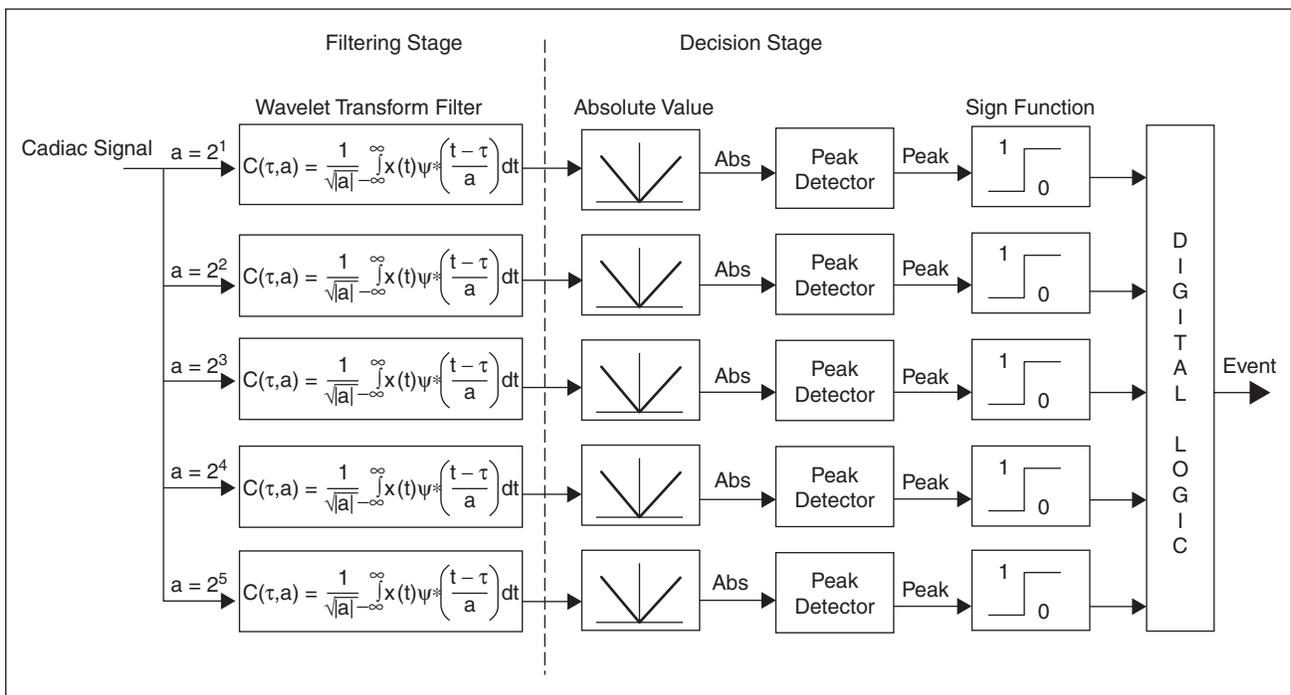
Fig. 13. Block diagram of the wavelet system.
