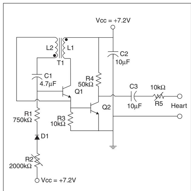
Fig. 5. A schematic of the first implanted pacemaker.
