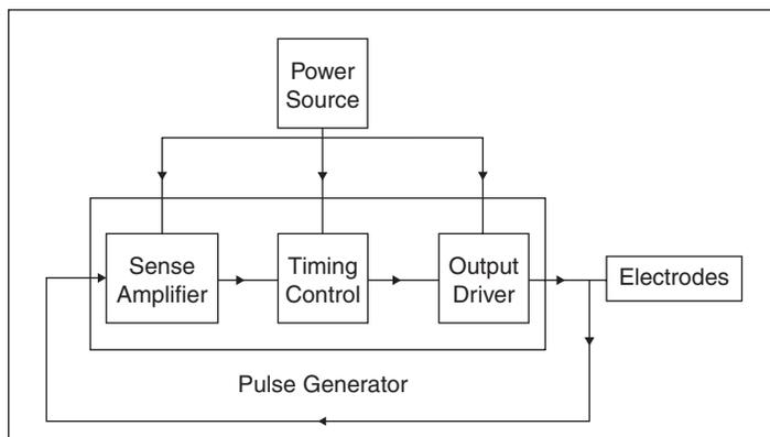
Fig. 6. Basic demand pacemaker functional block diagram.
