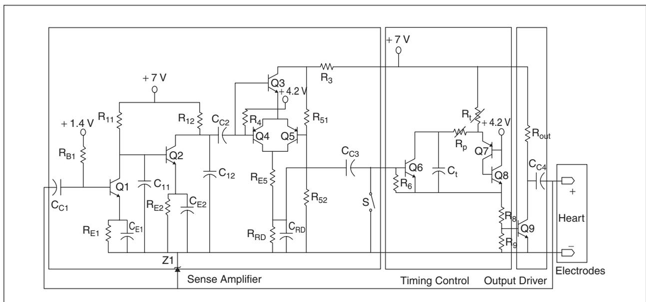
Fig. 7. A schematic of the pulse generator of the first demand pacemaker.
