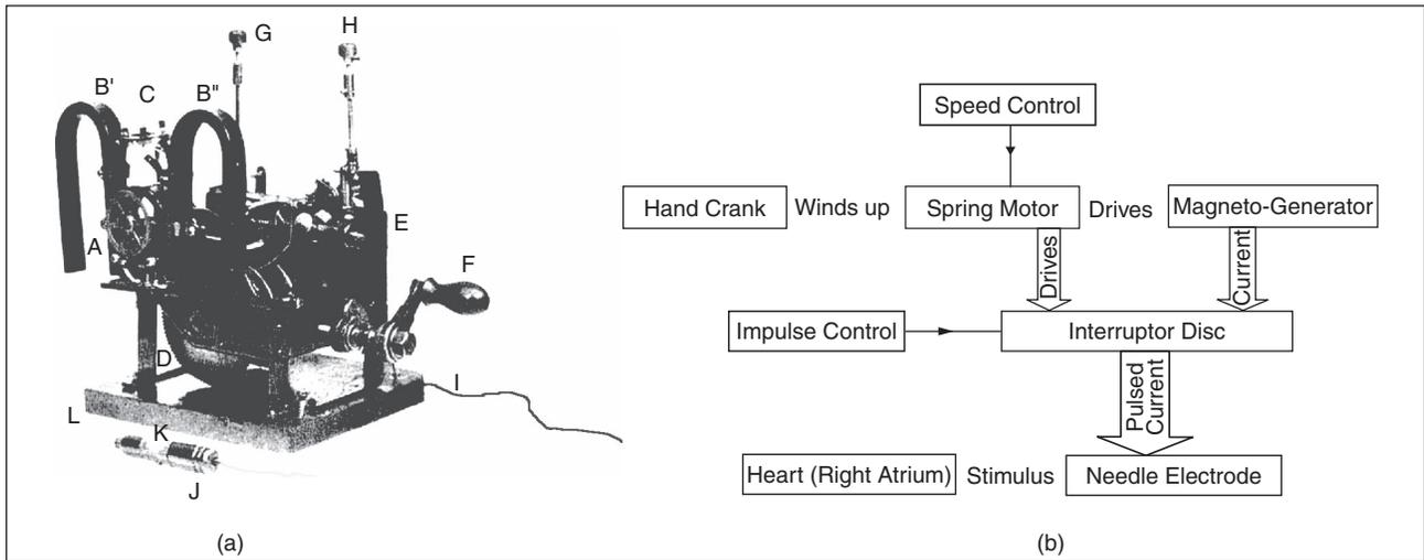
Fig. 4. (a) The first artificial pacemaker by Hyman. (b) Block diagram of Hyman's pacemaker.
