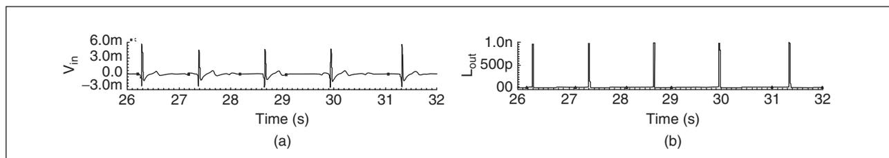
Fig. 11. Transient response of the complete sense amplifier circuit: (a) input voltage and (b) output current.
