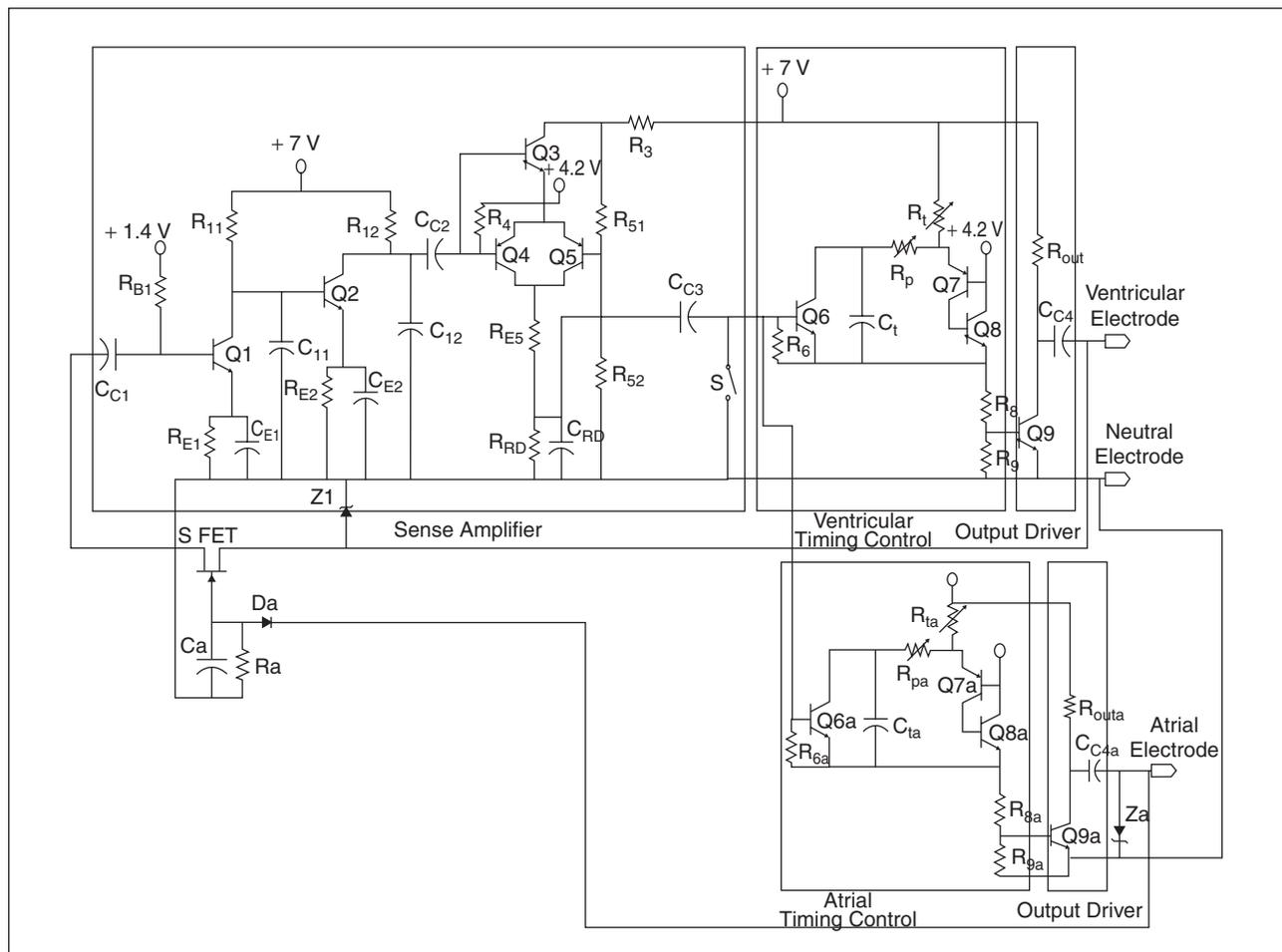
Fig. 8. Schematic of the dual-chamber demand pacemaker.
