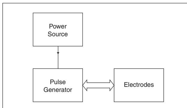
Fig. 3. Basic pacemaker functional block diagram.
