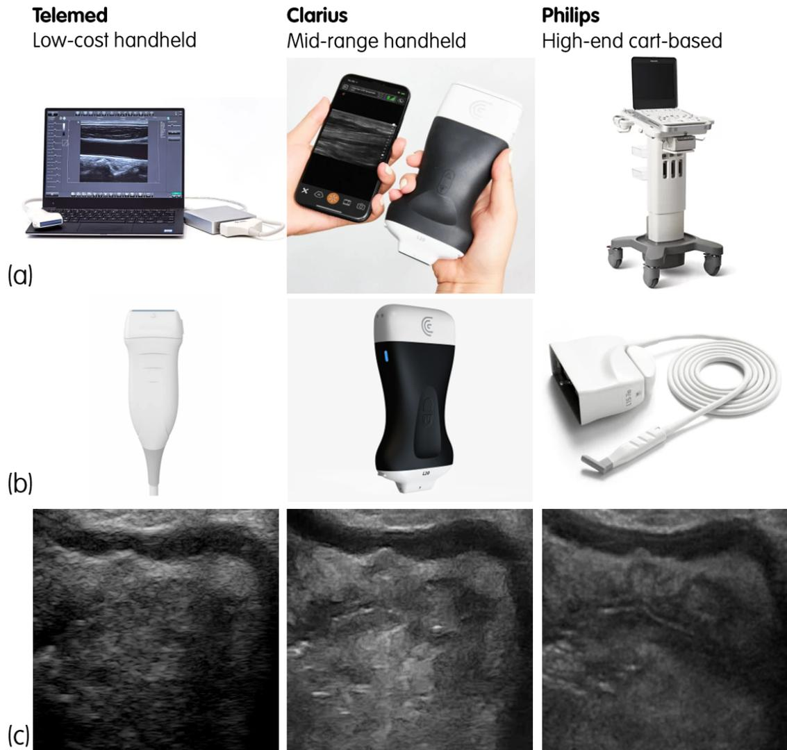
**Figure 2.1:** (a) Ultrasound devices used in this thesis, listed in increasing order of image quality: a cost-effective handheld device (Telemed), a mid-range handheld device (Clarius), and a high-end cart-based device (Philips). (b) Transducer used with each device. (c) Example ultrasound images acquired with each device.
