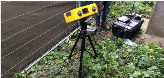
Figure 6.24: Interferometric radar station
