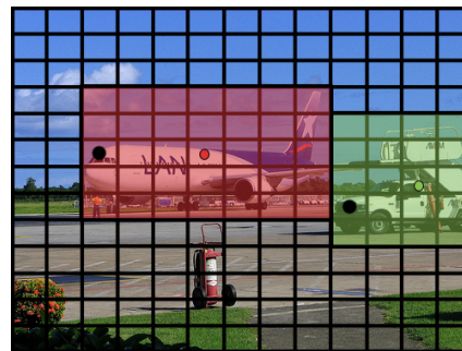
Figure 4-12: Illustration of free ground truth cell selection. The red and green points, represent the cells where the center points of each object resides. The black points represent which region the network might select when given a free choice.
