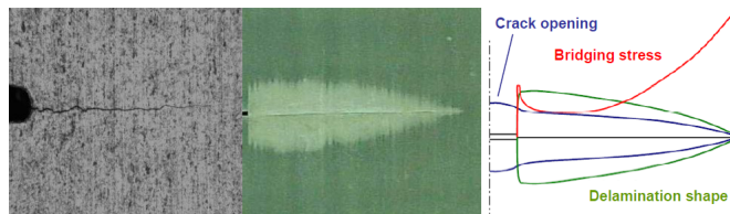
Figure 2.12: Crack in metal layer, delamination area and schematic view of crack [3, 21].
