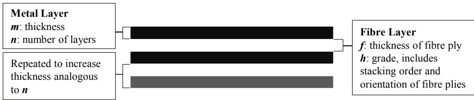
Figure 4.5: Lay-up definition of FML.
