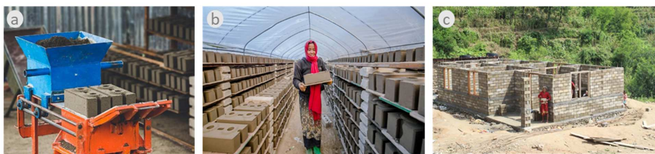
Figure 10. CSEB in Nepal; (a) compression press and ISSB, (b) curing of ISSB, (c) construction with ISSB. Sources: Community Impact Nepal.
