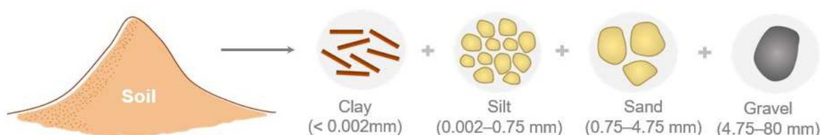
Figure 2. Composition of earth or soil based on ISO14688-2019, a guideline that specifies rules for identification and classification of soil. The aggregates of soils are represented with their size ranges as suggested in ISO14688-2019 [14]. Source: Kulshreshtha.
