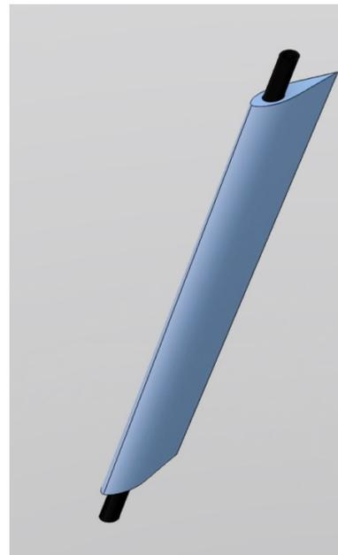
Figure 11.3: 3D Drawing of a single strut. The black pipe represents the carbon fibre rod, the blue shape indicates the EVA airfoil.
