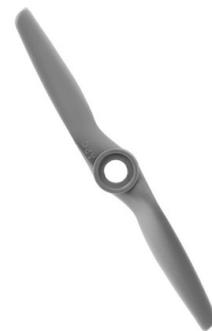
Figure 9.17: APC 4.1x4.1E Propeller
