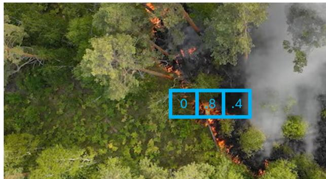
Figure 10.7: Example of camera view for illustrative purposes, with assigned risk scores for three  $10 \times 10$  m example patches. Aspect ratio (AR) does not represent the actual AR of the visual camera,
