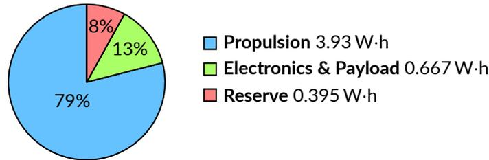
Figure 9.30: Energy Budget for Target 10-Minute Cruise Flight. Total Usable Battery Energy: 4.995 W-h
