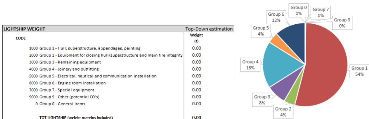
Figure 9: Top-down estimation in the weight sheet with the corresponding percentages of LSW per group
