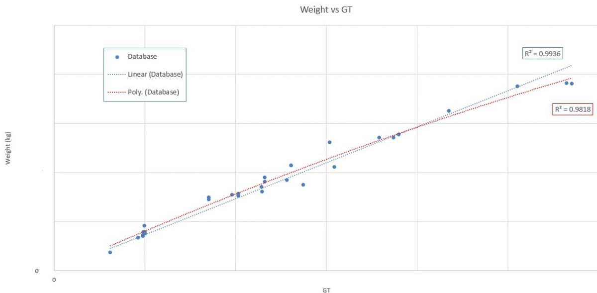
Figure 4: Example of a chart to estimate the weight converted from the GT based on a database of yachts
