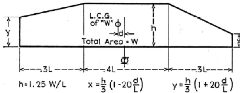
Figure 5: An approximation method for longitudinal weight distribution (Hansch, 2008)
