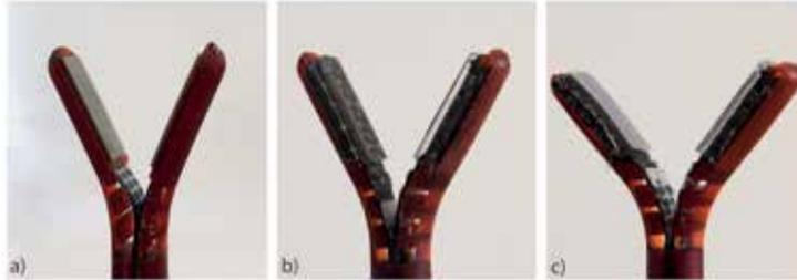
**Figure 6.4.** The three fabricated grippers. The reference gripper (a) was equipped with a grooved stainless-steel plate. In unpatterned pads (b), the elastomeric pads appear transparent, whereas in patterned pads (c), a white haze can be seen at the pad surface. In soft pads, either patterned or unpatterned, the CFF was embedded in the elastomeric pad.
