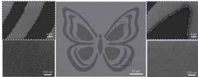
**Figure 2.5.** Electro-hydrodynamic jet printing of a butterfly from microdroplets of BCP solution. The light and dark colors originate from the use of two PS-*b*-PMMA, with different block sizes. The images left and right show magnifications of dark and light regions. The fingerprint-like patterns at the bottom two images are the result of BCP self-assembly. Reproduced with permission.<sup>[116]</sup> Copyright 2013, Springer Nature.
