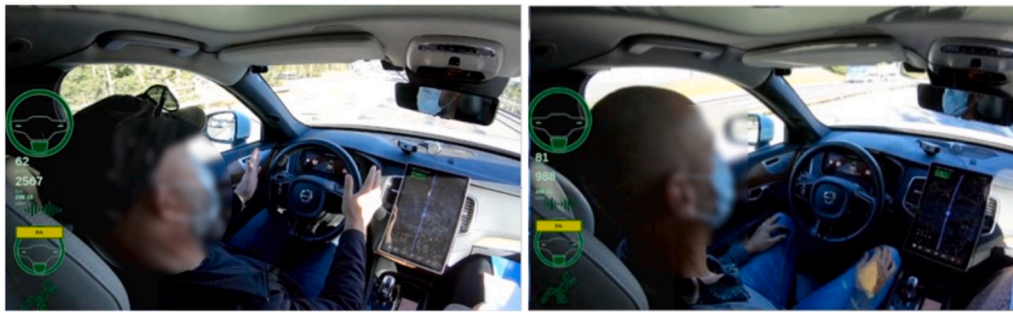
Fig. 4. Left: Driver testing the steering capability of the Level 2 driving automation; Right: Driver removing hands fully from the steering wheel during Level 2 driving automation.
