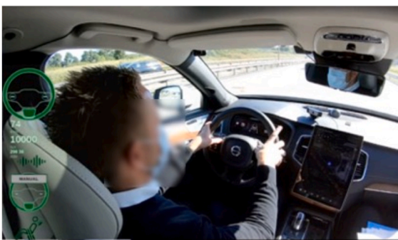
Fig. 3. The driver attempts to activate Level 3 using the steering wheel buttons in a situation where this mode is not available.
