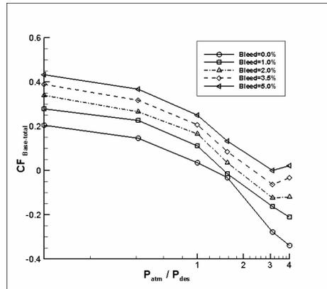
Figure 5: Total base thrust plotted against ambient pressure for different amounts of base bleed
