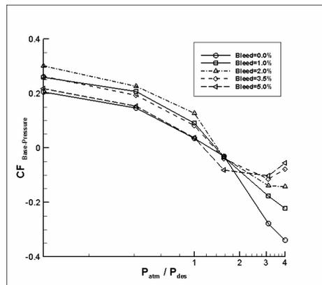
Figure 6: Base pressure thrust plotted against ambient pressure for different amounts of base bleed
