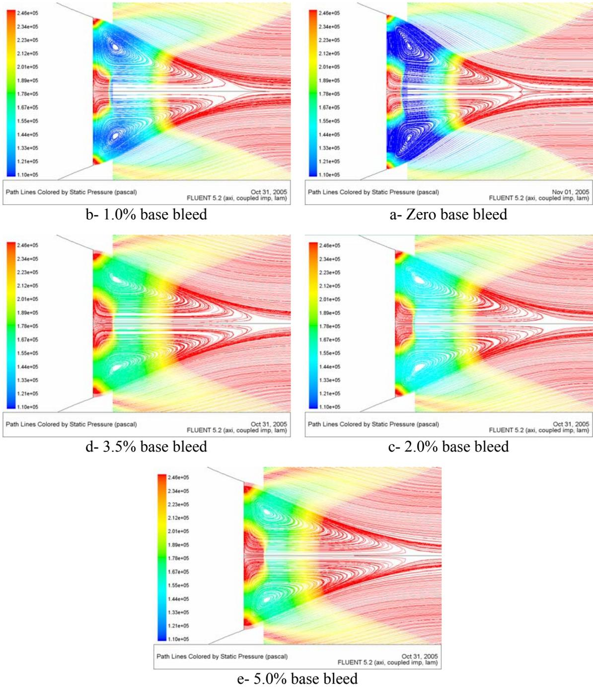
Figure 9: Pathlines colored by static pressure for different amounts of base bleed at  $P_{atm}/P_{des} = 4.0$
