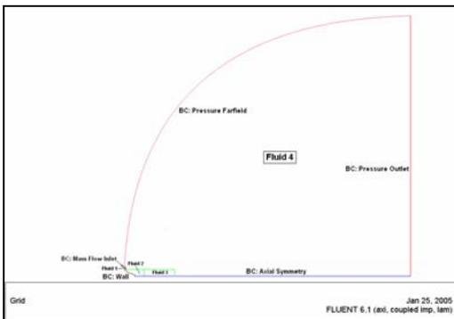
Figure 3: Numerical solution domain and boundary conditions
