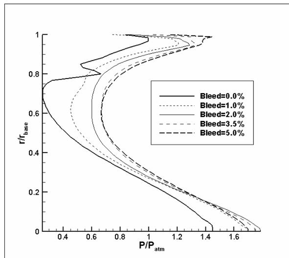
Figure 11: Base pressure distribution for different amounts of base bleed at  $P_{atm}/P_{des} = 4.0$
