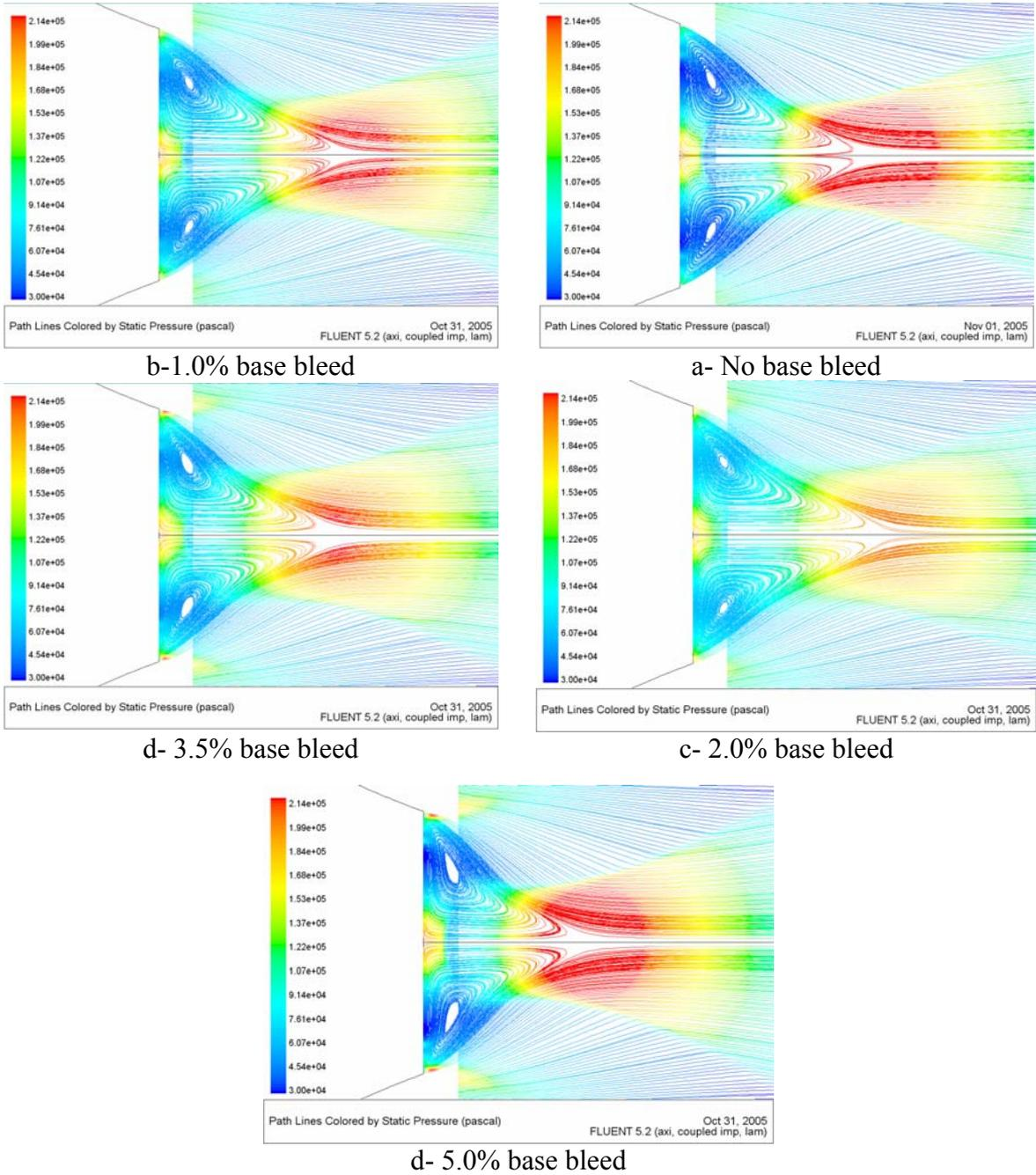
Figure 8: Pathlines colored by static pressure for different amounts of base bleed at  $P_{atm}/P_{des} = 0.1$
