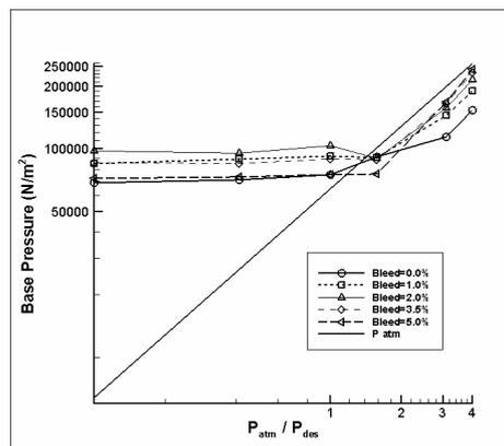
Figure 7: Average base pressure plotted against ambient pressure for different amounts of base bleed
