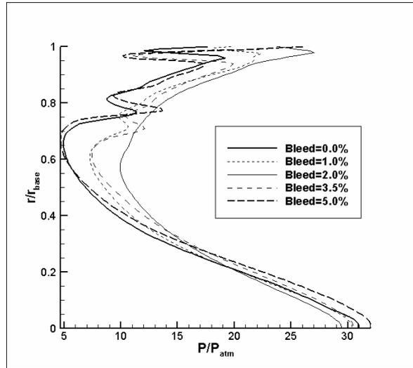
Figure 10: Base pressure distribution for different amounts of base bleed at  $P_{atm}/P_{des} = 0.1$
