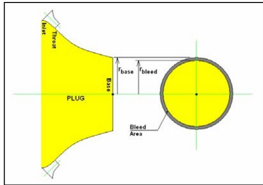
Figure 2: Geometry of truncated plug with base bleed
