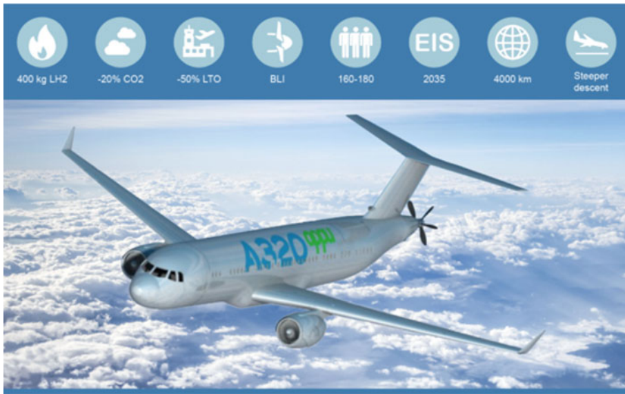
Figure 1. Rendering of the A320 APPU with key characteristics [16].
