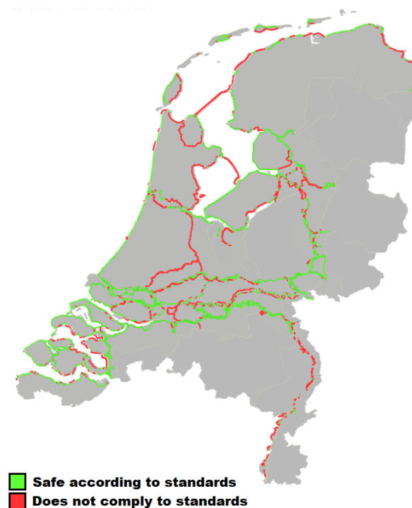
Figure 1.1: Assessment of flood defense structures
