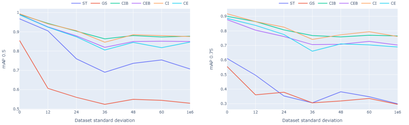
Figure 3: The Mean Average Precision results of Experiment 3. The left figure shows the mAP measurements for an IoU of 0.5 and the right figure shows the mAP measurements for an IoU of 0.75. The standard Faster R-CNN (ST and GS) models show a significantly stronger decrease in efficiency compared to the architectures with the CEConv layers (CIB, CEB, CI, and CE).
