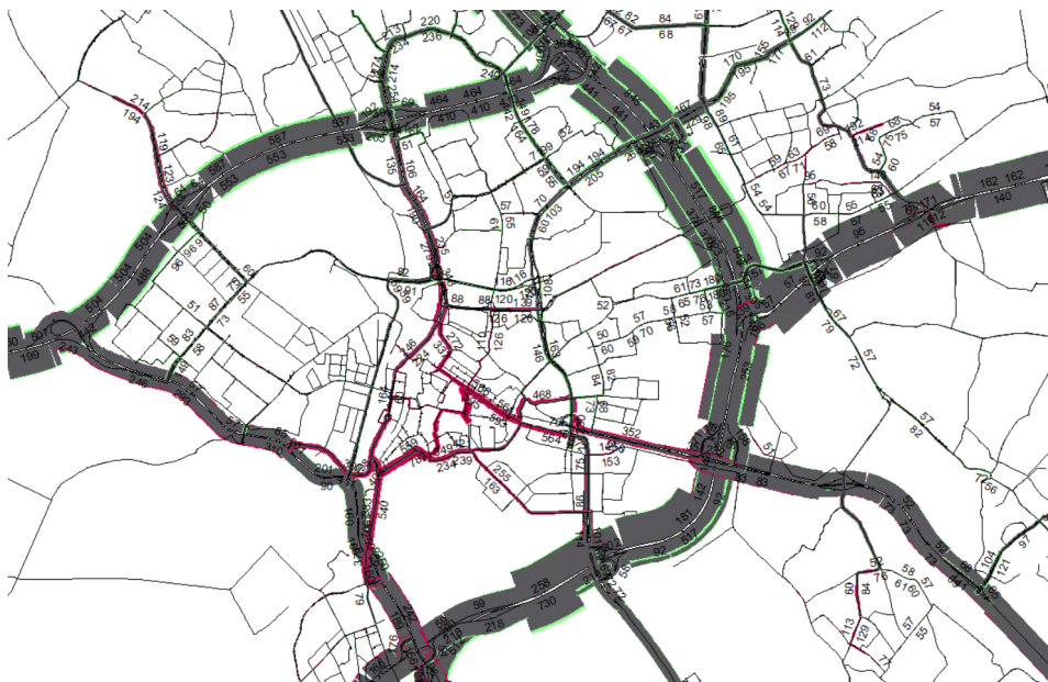
Figure B.12: Difference in intensities for the trip purpose Socrec between model A2 and B2. Red: A2 < B2 , Green: A2 > B2
