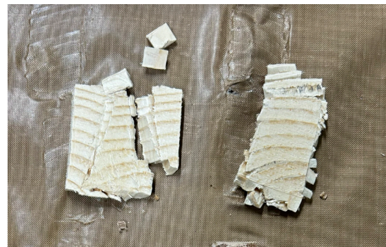
Figure 4.18 Two-layered sample of 1 cm veneers shattered in press.
