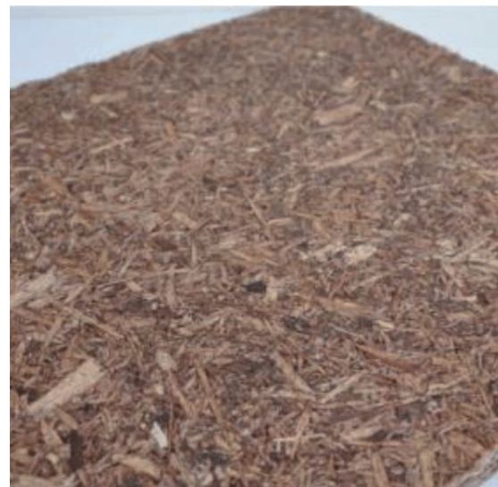
Figure 1.4 Particleboard produced with tannin-based adhesives. From Zhou & Du, 2019. Licensed under Creative Commons Attribution 3.0 Unported.
