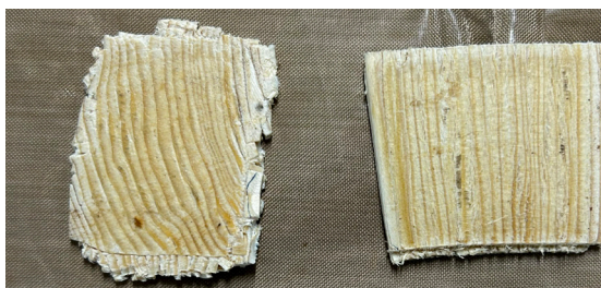
Figure 4.17 Cross-grain (right) sample shows extreme expansion compared to the end-grain (left).
