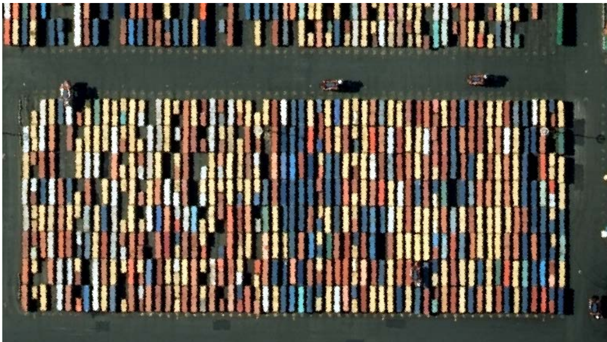
Figure 4.34: Example: ladens stack operated by straddle carriers (aerial imagery by the National Georegister (NGR) is licenced under CC BY 4.0).
