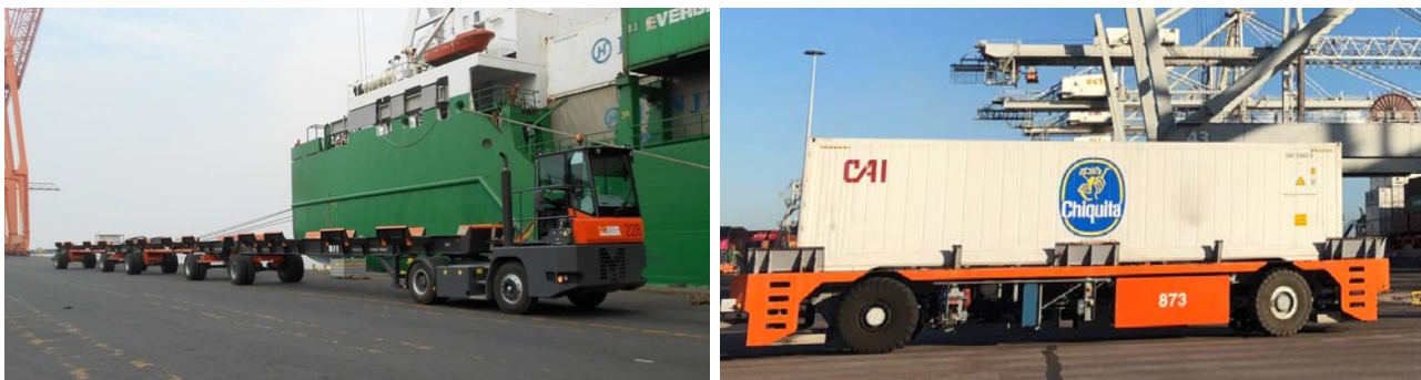
Figure 4.20: Container transport vehicles; left: Multi Trailer System (MTS) (by Govender et al., 2017 , is licenced under CC BY 4.0); right: Automated Guided Vehicle (AGV) (by Europe Container Terminals (ECT) is licenced under CC BY-NC-SA 4.0).
