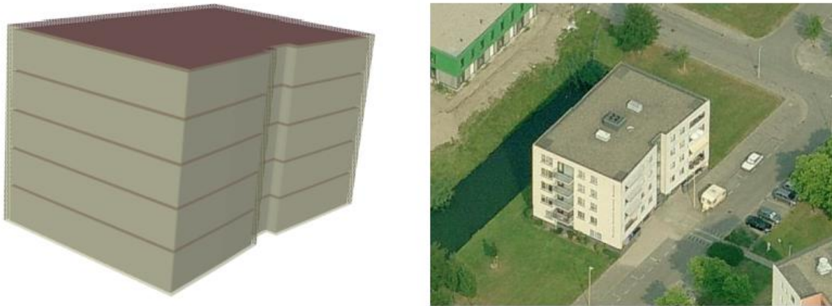
Figure 8: Example of a LOD2+ buildings with indoor information about floors (left) and the he same building in reality (right)
