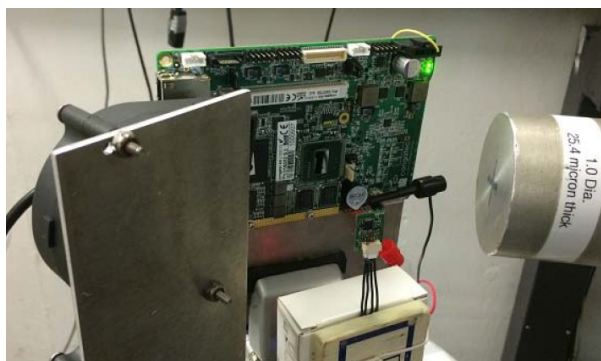
(a) A Conga QA6 - Intel E620 testing board at a radiation facility [40].
