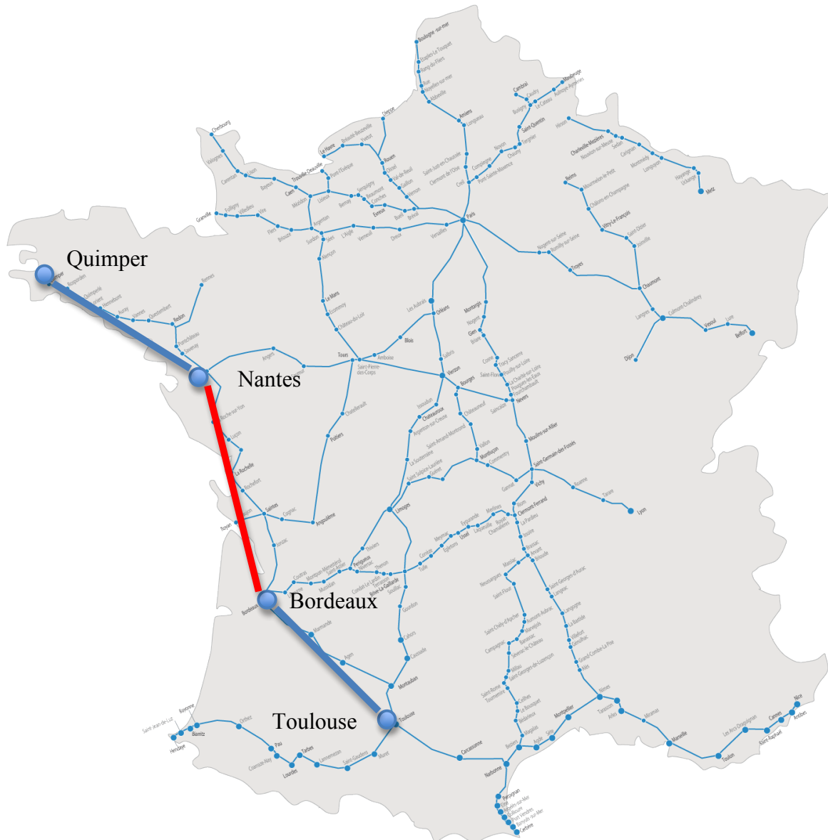
Figure 7: Quimper-Nantes-Bordeaux-Toulouse Intercity line. In red the section partially not electrified
