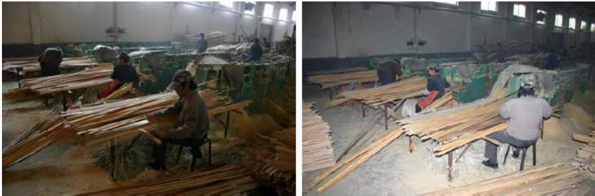
Figure 10 – Rough planing of bamboo strips (Van der Lugt, 2008)
