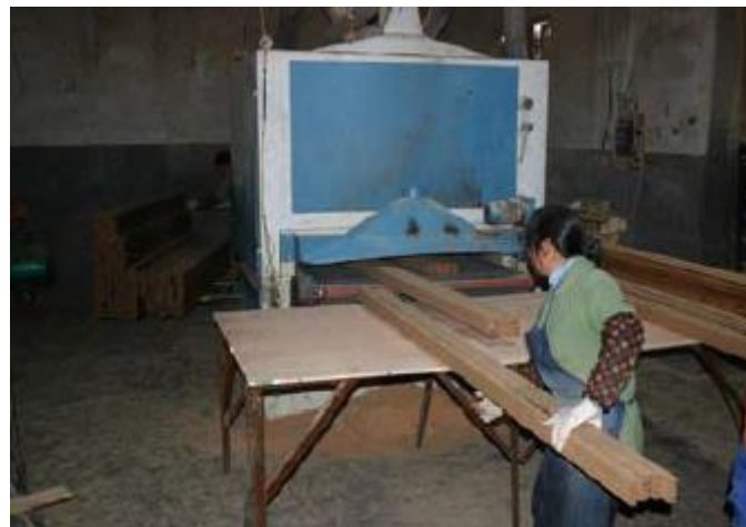
Figure 17 – Multi-layer cold press (Van der Lugt, 2008)
