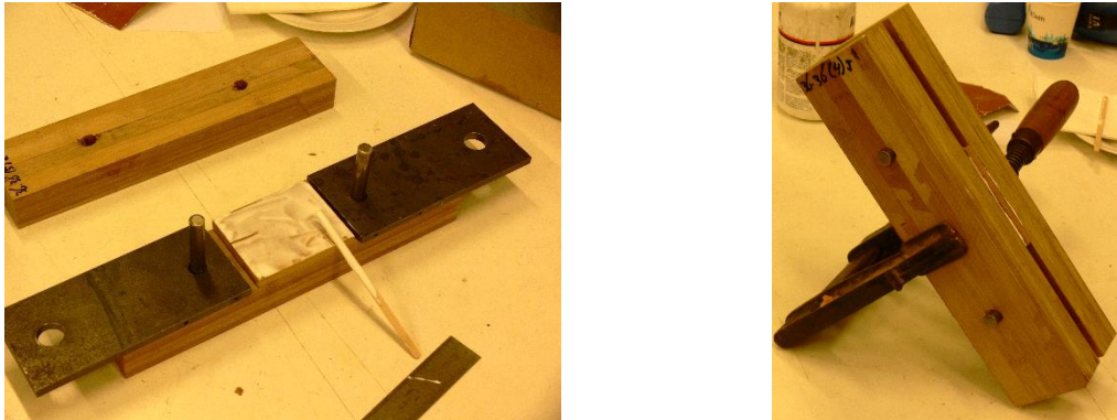
Figure 63 - Gluing process using a PVAc wood glue
