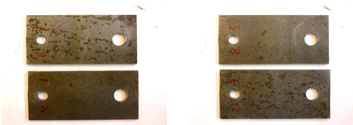
Figure 64 - Embedment deformation of the slotted-in steel plates
