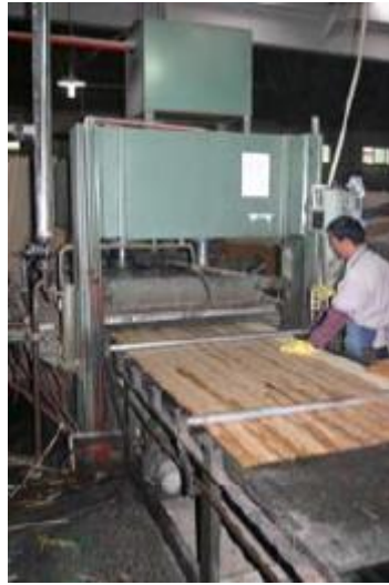
Figure 16 – Hot pressing of 1-layer bamboo boards (Van der Lugt, 2008)
