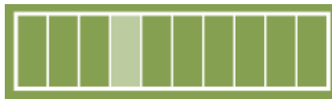
Figure 14 – Side Pressed (SP) (MOSO International BV, 2016)
