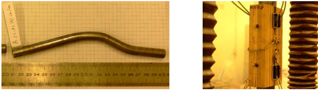
Figure 65 - Asymmetrical bending of the dowel
