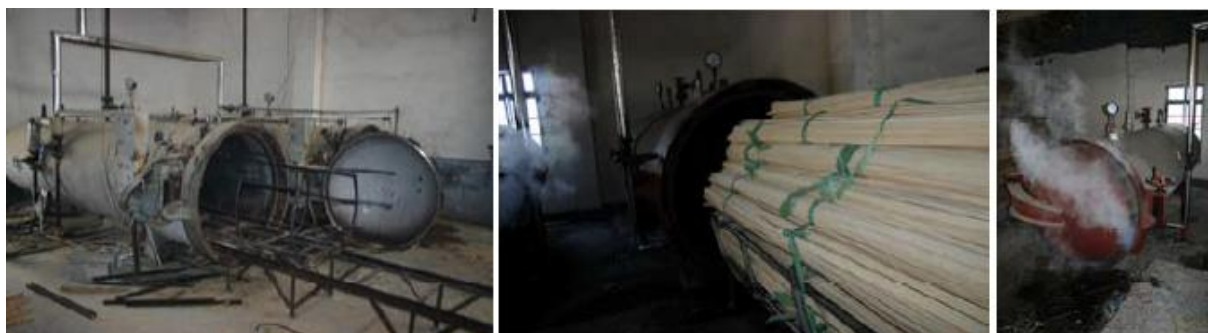
Figure 12 - Carbonization process (Van der Lugt, 2008)
