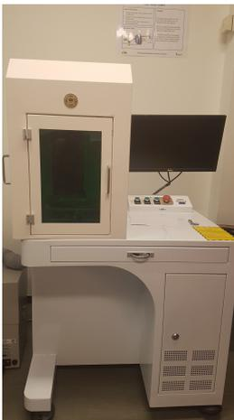
(a) Laser cutter set up
