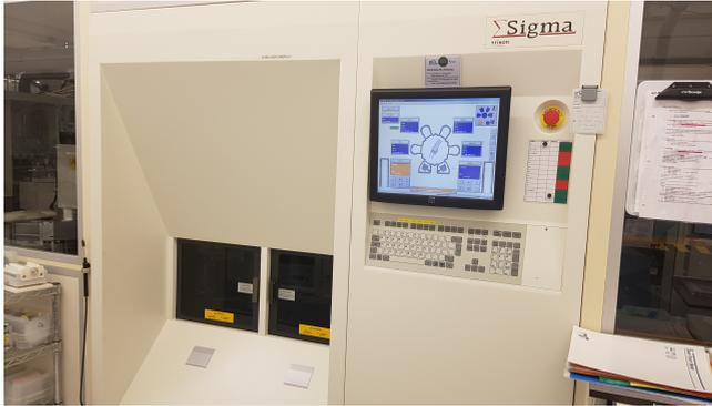
Figure E.4: Metal sputtering equipment in EKL lab
