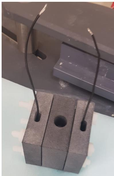
Figure 2.3: Isometric view of assembled Si-air cell
