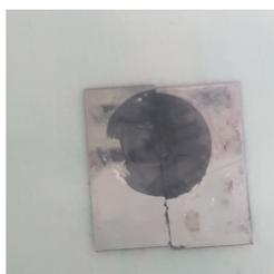
Figure 7.1: Broken Si sample.
