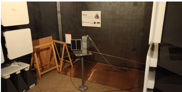
(a) Measurement setup for radiated emission test
