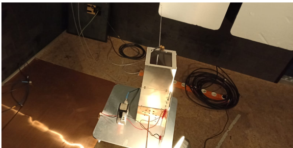
(a) Measurement setup for conducted emission test
