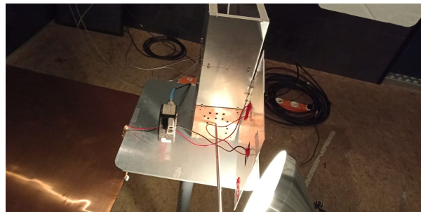
(b) Measurement setup for conducted emission test
