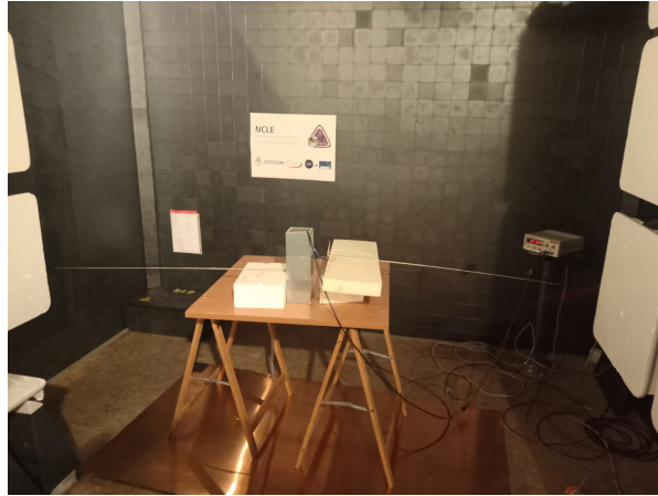
Figure B.5: Lab test with DC-DC converter, antenna and low noise amplifier integrated in cubesat.
