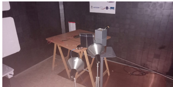
(b) Measurement setup for radiated emission test with light source for solar panels
