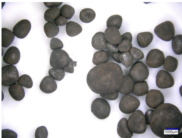
Figure 7. Sand grains covered in manganese oxides (black) from drinking water treatment plant Holten (Vitens N.V). Picture courtesy of Simon Muller.
