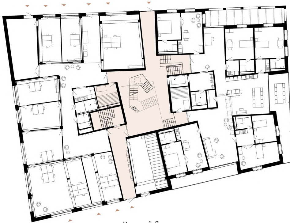
Ground floor access to workspaces and dwellings from east-west facade
