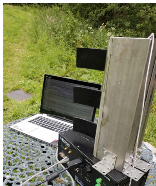
Figure 1. The FOSS Sensor with the three fins, each containing a FBG sensor
