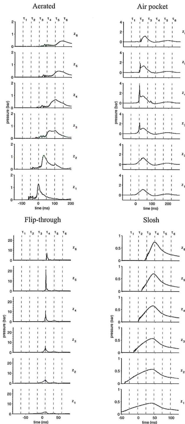
Fig. 31 Pressure time series along centreline of concrete block for aerated, air pocket, flip-through and slosh impact
