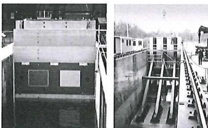
Fig. 9 Test wall as installed in Delta flume
