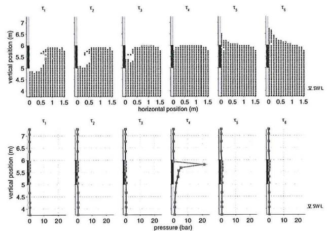
Fig. 29 Flip-through impact (test 74), wave shape and pressure profile at 6 time instants, maximum pressure at  $\tau_4$  and  $\Delta\tau = 25$  ms
