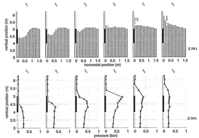
Fig. 30 Slosh (test 24), wave shape and pressure profile at 6 time instants, maximum pressure at  $\tau_4$  and  $\Delta\tau = 25$  ms
