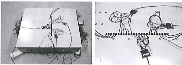
Fig. 24 Primary NO96 box with external accelerometers
