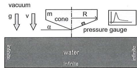
Fig. 18 Verification conditions of pressure sensors
