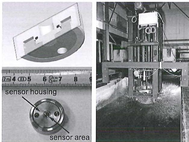
Fig. 19 Pressure gauge including housing and shooting apparatus
