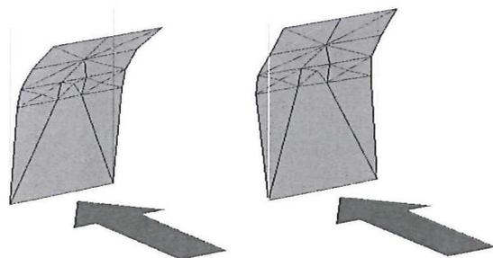
Fig. 23 Test wall's first and second vibration modes
