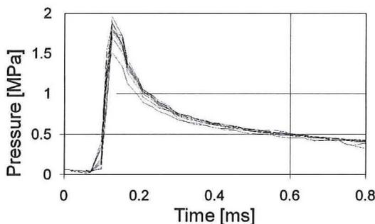
Fig. 20 Cone pressures recorded in 10 different tests
