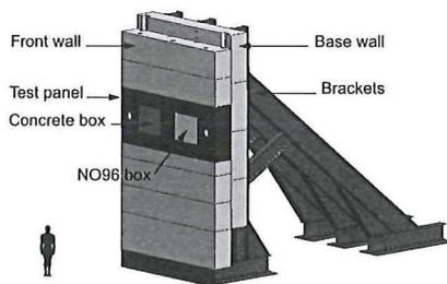
Fig. 8 Test wall design
