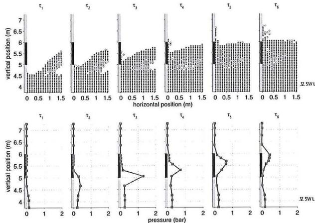
Fig. 27 Aerated impact (test 86), wave shape and pressure profile at 6 time instants, maximum pressure at  $\tau_3$  and  $\Delta\tau = 50$  ms
