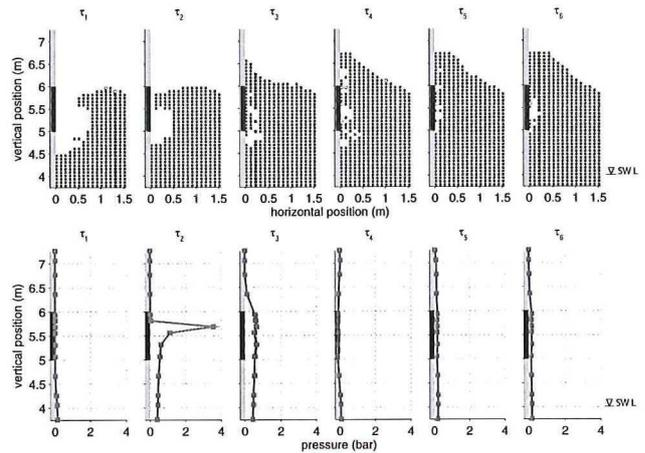
Fig. 28 Air pocket impact (test 79), wave shape and pressure profile at 6 time instants, maximum pressure at  $\tau_2$  and  $\Delta\tau = 50$  ms
