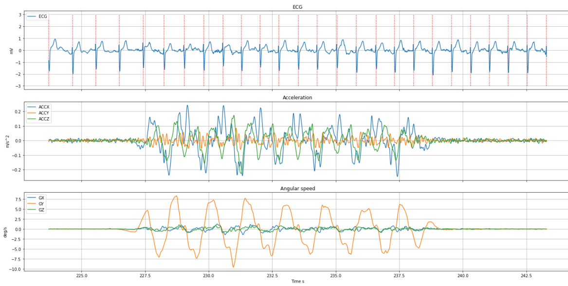
Figure 41. ECG, acceleration, and angular speed recorded with the wearable device while performing torso rotations.
