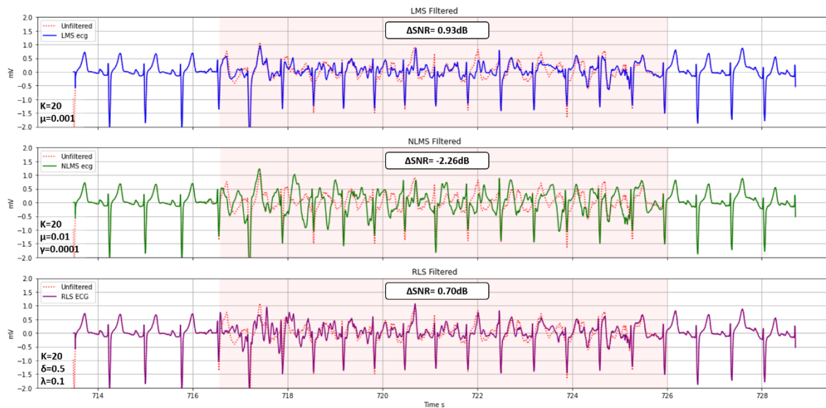
Figure 31. Filter output using the recomposed reference input after being processed with the wavelet transform method.
