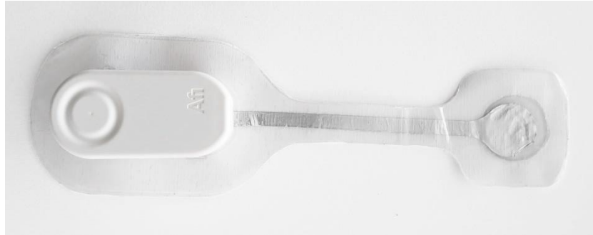
Figure 2. Single-lead ECG Wearable device AFi ® with a self-adhesive Ag/Cl electrode.
