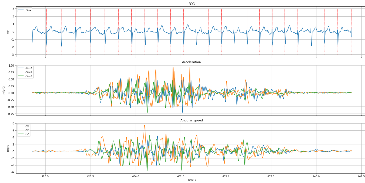
Figure 43. ECG, acceleration, and angular speed recorded with the wearable device while walking.
