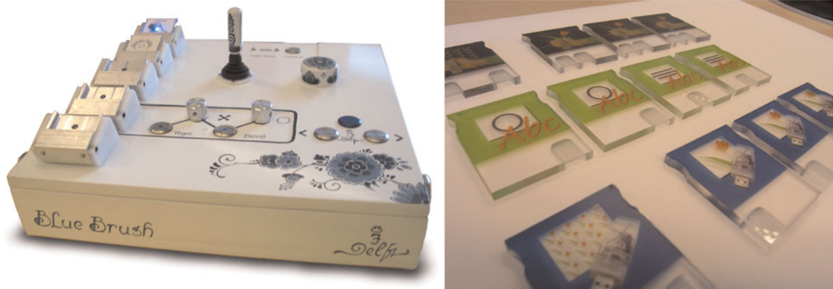
Fig. 10. The Bluebrush panel consists of a tangible, dedicated interface for designing Delft blue earthenware. The left side of the panel houses slots for media, and the right side of the panel houses various controls to manipulate the media. Media are loaded into a layer by inserting a token (right) into the corresponding slot. There are tokens for the various media types: images captured with a webcam, texts, and collections of images, for instance, from a USB flashdrive. [A color version of this figure can be viewed online at journals.cambridge.org/aie ]
