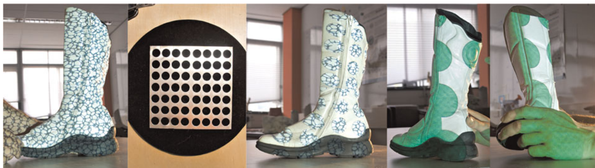
Fig. 6. Examples of “skinned” objects. (Left) An object with a digital pattern. (Center) A physical material and the object skinned with both the digital pattern and the physical material. Notice the deformation in the circle patterns. (Right) Two examples of object manipulation that alter the location and orientation of the projected pattern. [A color version of this figure can be viewed online at journals.cambridge.org/aie ]
