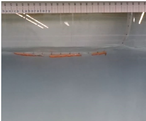
(c) When the velocity increase to one limitation or when the water surface level decrease, the proxy get to a horizontal position and moving with water surface
