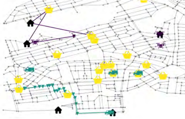
Figure 3.2: A cutout of one particular state of the simulation is illustrated. The road network graph, on which trucks move is shown in grey. The plans of one drone and one truck are highlighted in purple and green. Goal locations of known and non-delivered orders are shown in yellow.
