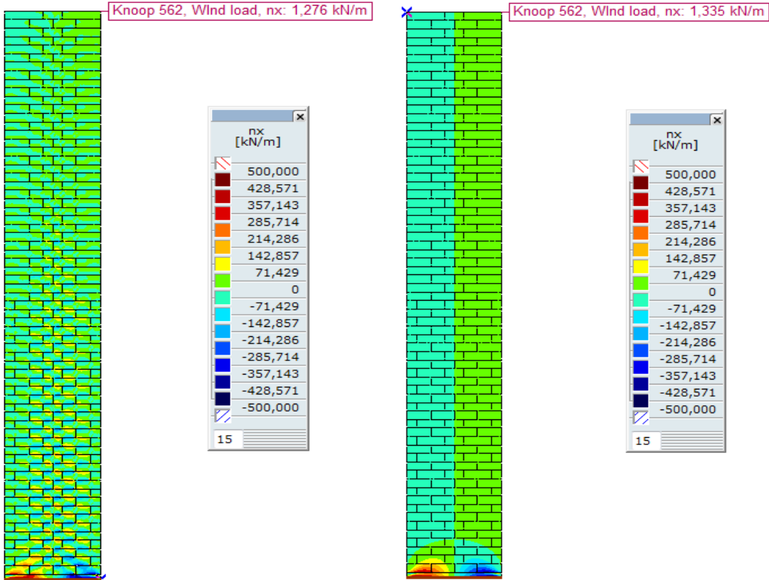
Figure 149 Load introduction of the floors in a precast (left) and monolithic (right) 2D model
